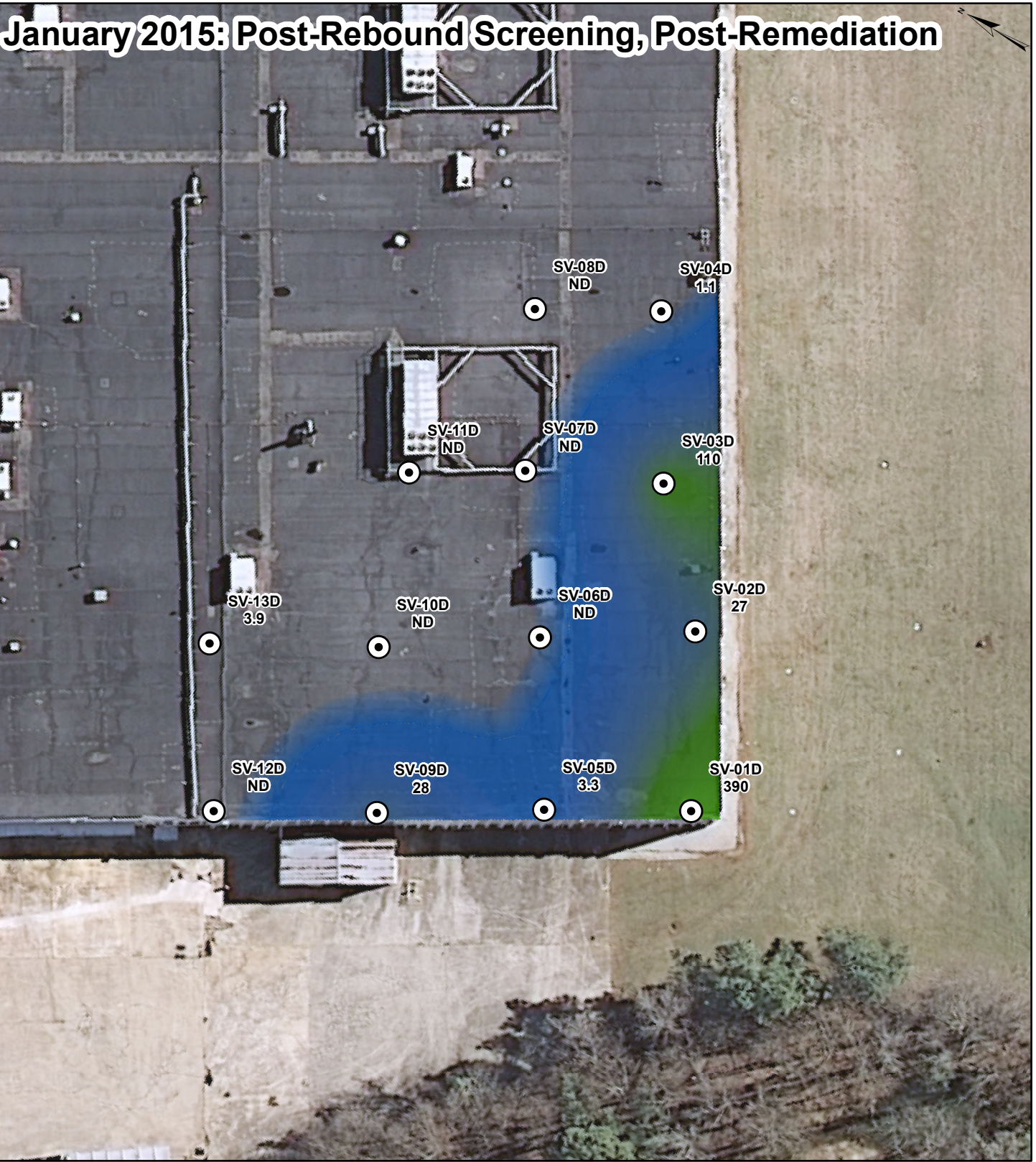
FIGURE 4-5C: 1,1-DCA IN DEEP SOIL GAS 2007 VS. 2015 CONCENTRATIONS ( \mu\text{g}/\text{m}^3 ) FORMER AVERY DENNISON PROPERTY FLOWERY BRANCH, GEORGIA
