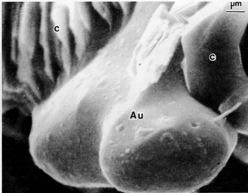
Figure 31. SEM photomicrograph showing spheroidal gold (Au) as commonly seen in the vicinity of covellite (c), Parks Mine.
