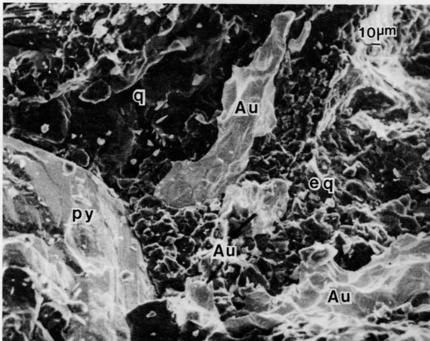
Figure 25. SEM photomicrograph showing irregularly shaped gold (Au) in strongly etched quartz (eq) and near slightly altered pyrite (py), Parks Mine. Quartz (q).
