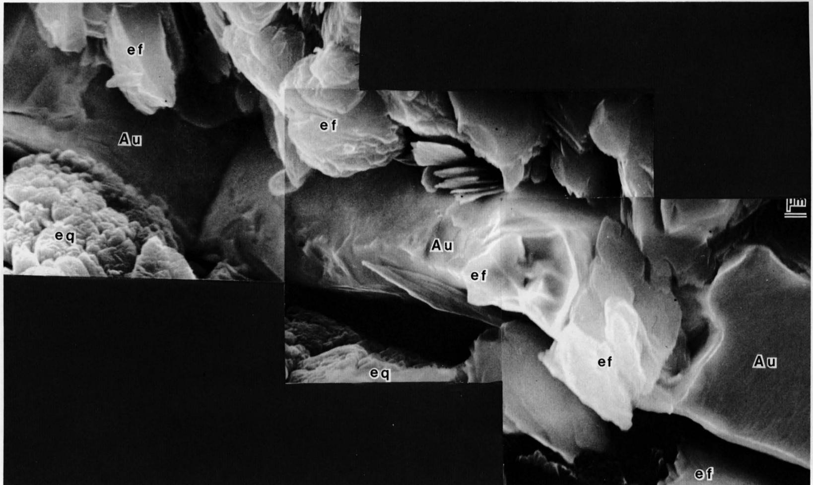
Figure 20. SEM photomicrograph showing typical distribution of gold (Au) along an etched micro-fracture in vein quartz, Parks Mine. Etched quartz (eq), etched K-feldspar (ef).
