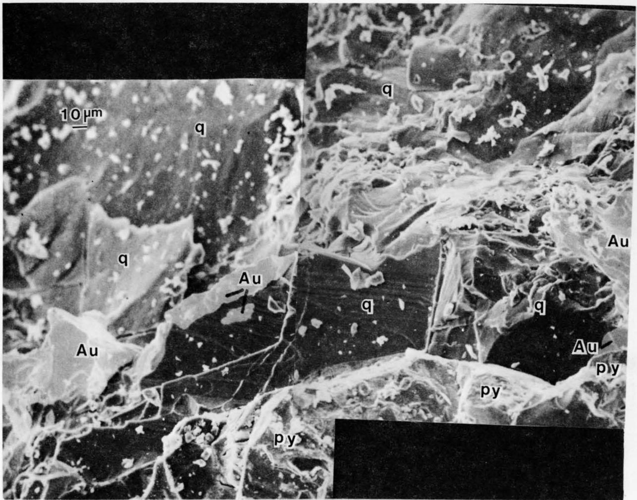
Figure 23. SEM photomicrograph showing auriferous (Au) micro-fracture in vein quartz (q), Parks Mine. Pyrite (py).
