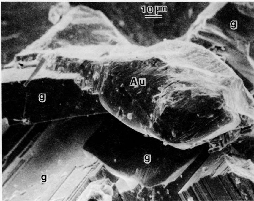
Figure 32. SEM photomicrograph showing gold (Au) in contact with partially altered galena (g), Parks Mine.
