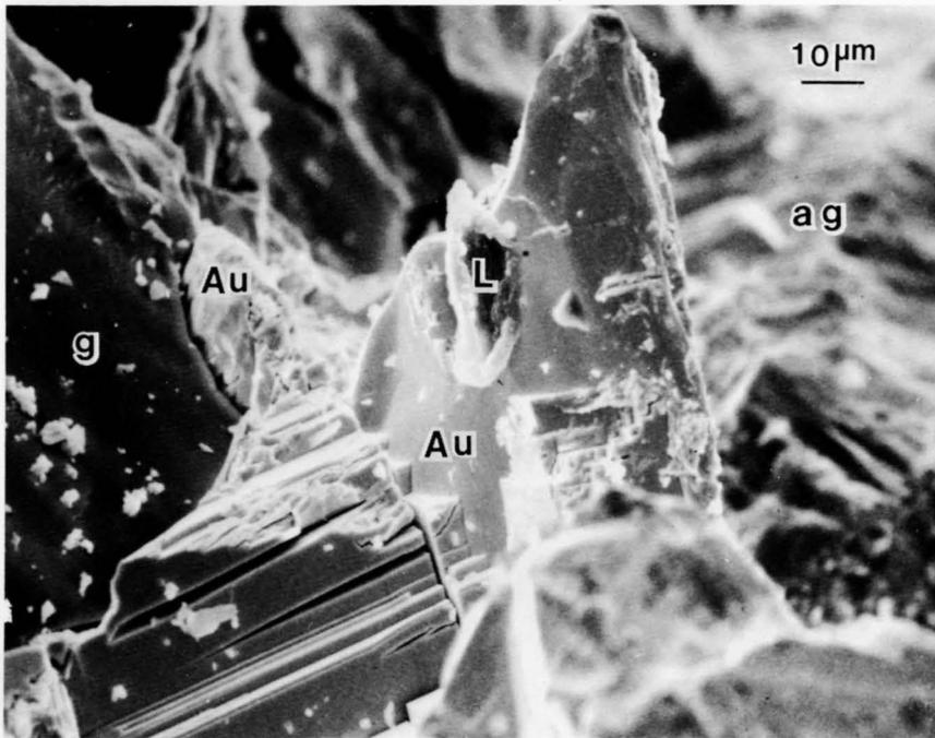
Figure 34. SEM photomicrograph showing gold (Au) in planar contact with apparently unaltered galena (g) and in contact with altered galena (ag), Parks Mine. Limonite (hematite-goethite) (L).
