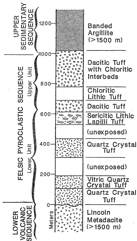
Figure 2. Representative stratigraphic section of the Little River series at the headwaters of Wells Creek near Lincolnton, Georgia (from Whitney, et al., 1978).
