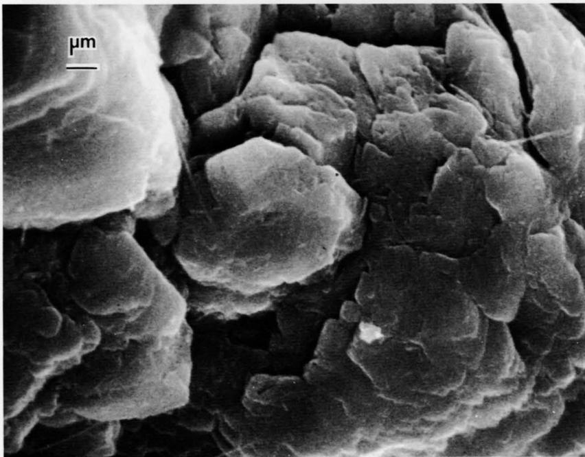
Figure 15. SEM photomicrograph showing etched quartz crystals along a micro-fracture in vein quartz, Parks Mine.
