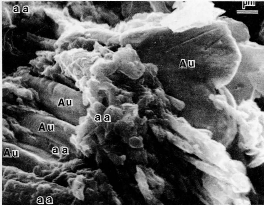
Figure 45. SEM photomicrograph showing alternating tabular masses of gold (Au) and amphibole (aa), Latimer Mine.
