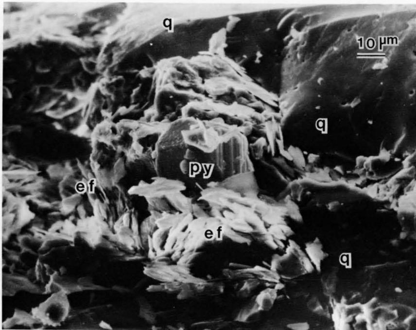
Figure 21. SEM photomicrograph showing euhedral, striated pyrite crystal (py) surrounded by etched K-feldspar (ef) and quartz (q) in a micro-fracture of vein quartz, Parks Mine.
