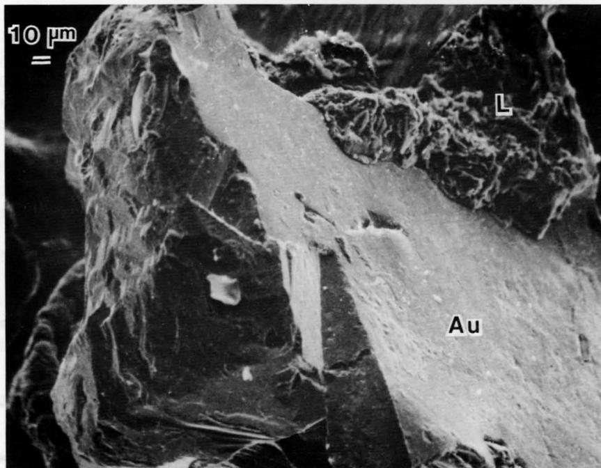
Figure 10. SEM photomicrograph showing large gold (Au) surface in contact with porous limonite (L) (pseudomorphous after pyrite), Landers Prospect.
