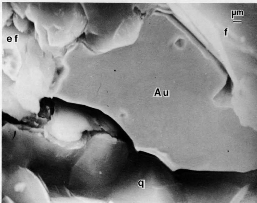
Figure 22. SEM photomicrograph showing gold (Au) in contact with highly corroded K-feldspar (ef) and quartz (q) along a continuation of the micro-fracture shown in Figure 21. K-feldspar (f).
