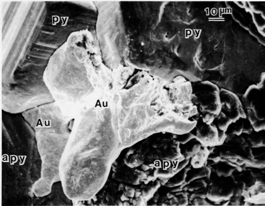
Figure 26. SEM photomicrograph showing gold (Au) in contact with striated and slightly altered pyrite (py) and with strongly altered pyrite (apy), Parks Mine.
