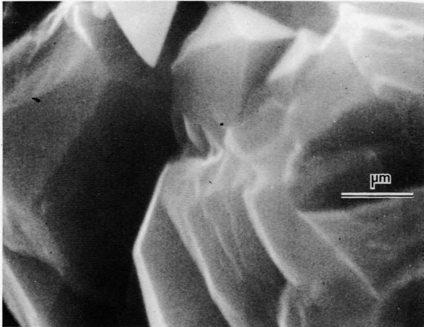
Figure 14. SEM photomicrograph showing small euhedral quartz crystals that have grown into micro-openings in vein quartz, Parks Mine.
