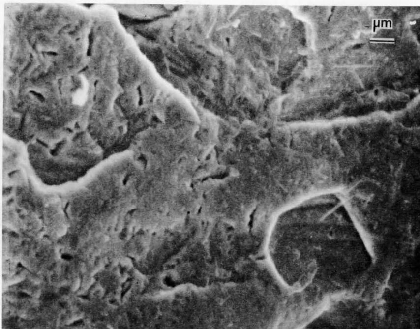
Figure 17. SEM photomicrograph showing surface of a gold particle that was deposited on, and now is a replica of, an etched quartz surface, Parks Mine.
