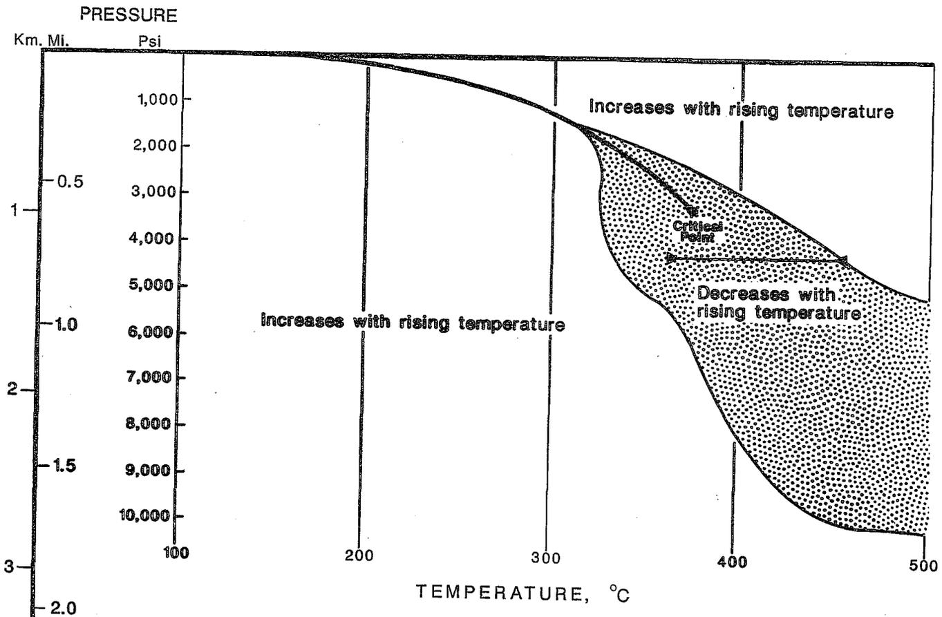
Figure 49. Temperature-pressure field within which the solubility of silica decreases with increasing temperature. The approximate temperature interval within which the solubility of quartz increases with decreasing temperature is indicated by the horizontal bar. Data from Hertman (1964) and Kennedy (1970).
