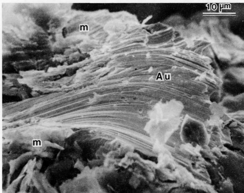
Figure 39. SEM photomicrograph showing gold (Au) altered mica (m), Parks Mine.
