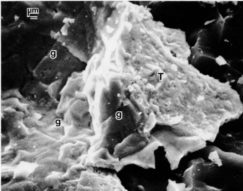
Figure 37. SEM photomicrograph showing gold-silver-telluride (T) associated with altered galena (g), Parks Mine.
