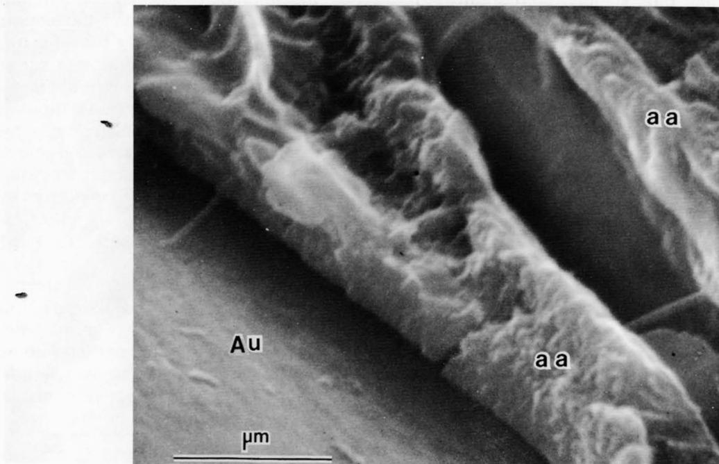
Figure 43. SEM photomicrograph showing close-up of goethitic septa, formed by alteration of amphibole (aa), in contact with gold (Au), Latimer Mine.
