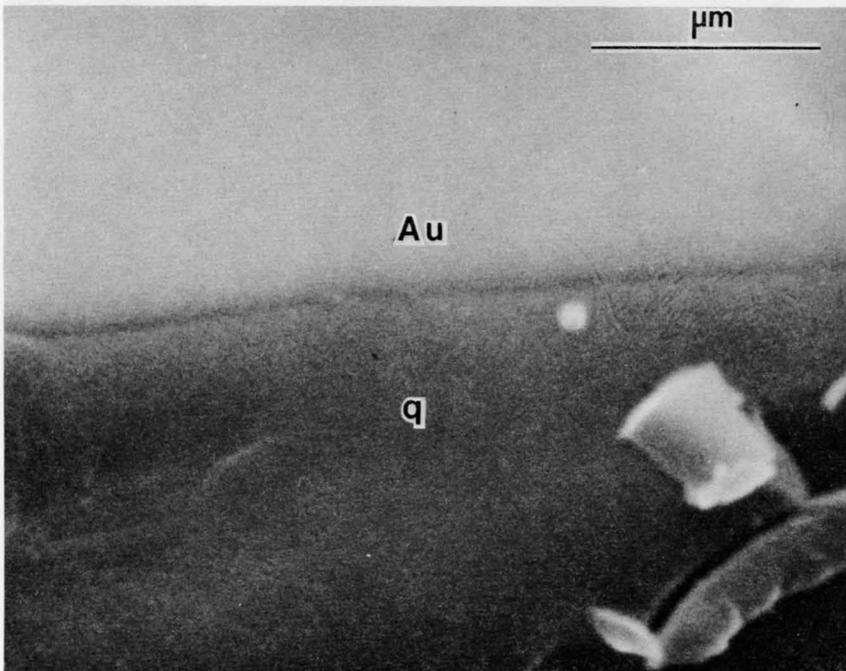
Figure 19. SEM photomicrograph showing gold (Au)- quartz (q) contact in vein quartz, Parks Mine.
