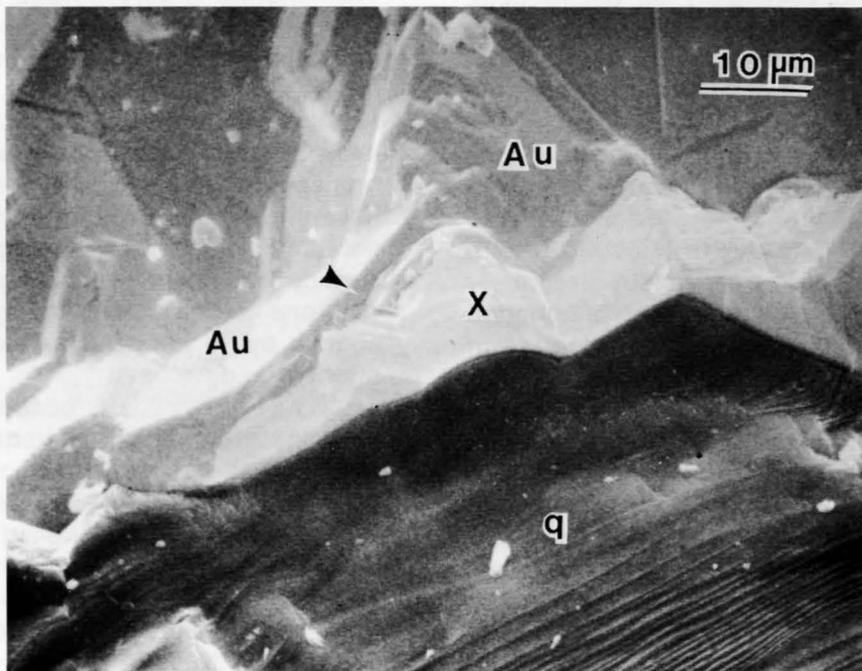
Figure 8. SEM photomicrograph showing auriferous silica (x) in contact with gold (Au) and quartz (q), Landers Prospect.
