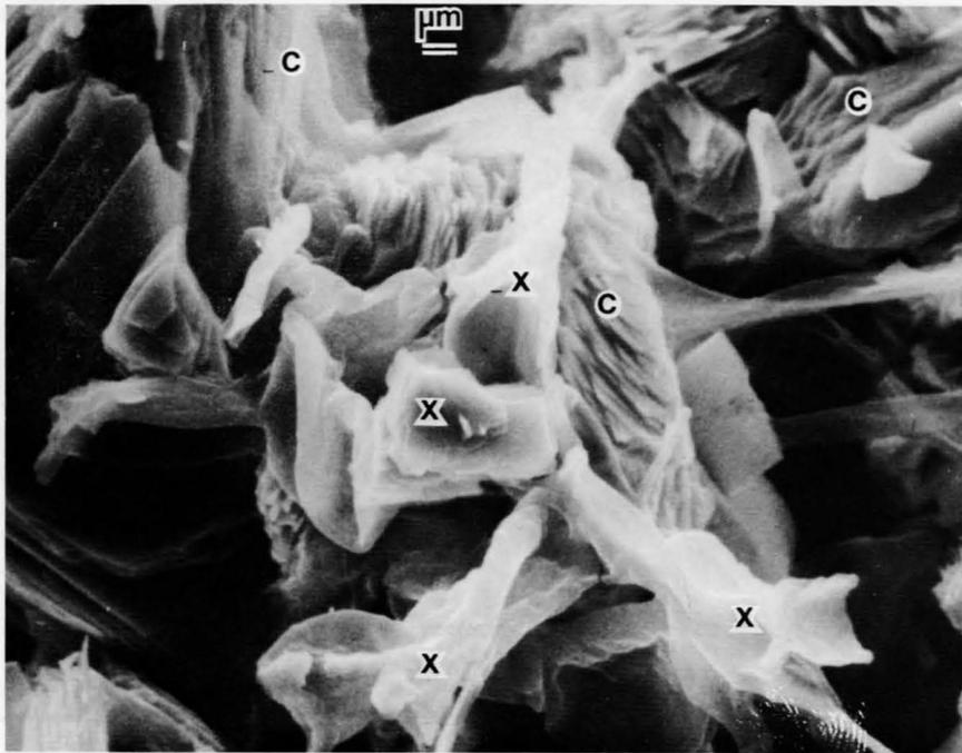
Figure 27. SEM photomicrograph showing covellite (c) etched along basal cleavage, Parks Mine. Sulfur-rich unidentified mineral (x).
