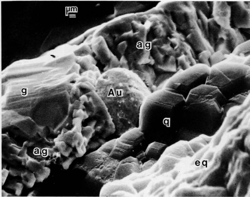
Figure 36. SEM photomicrograph showing gold (Au) in highly altered galena (ag) in vein quartz (q), Parks Mine. Galena (g), etched quartz (eq).
