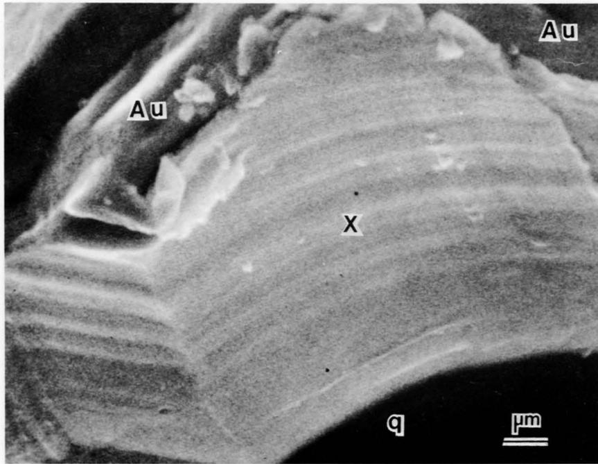
Figure 9. SEM photomicrograph showing enlargement of a portion of Figure 8. Gold (Au), quartz (q), auriferous silica (x).
