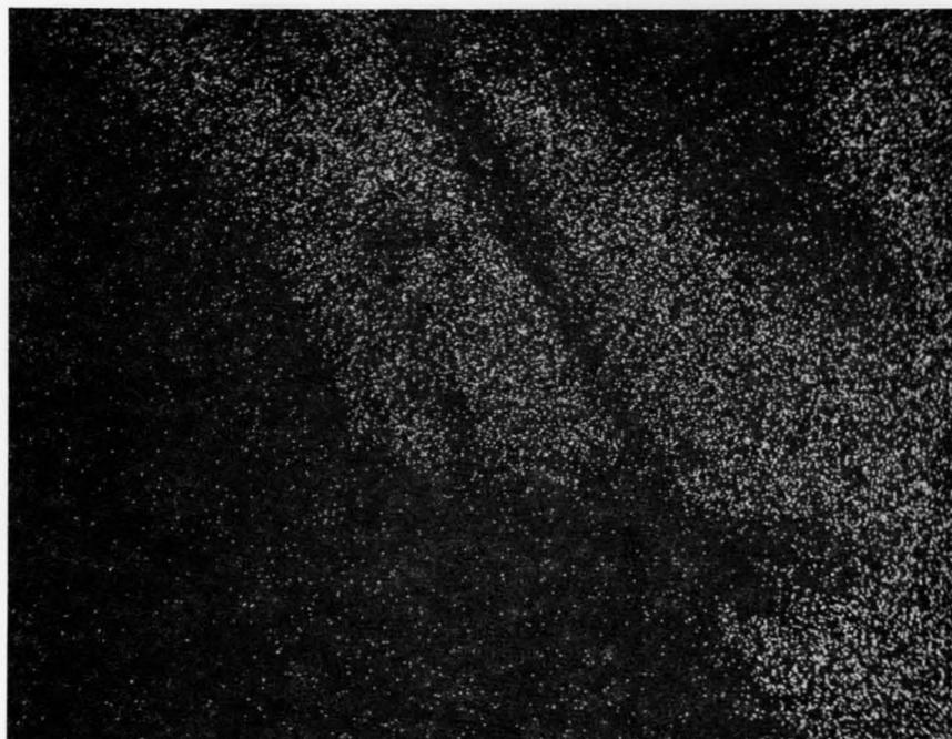
Figure 41. SEM photomicrograph showing X-ray map showing the distribution of gold in Figure 40. /
