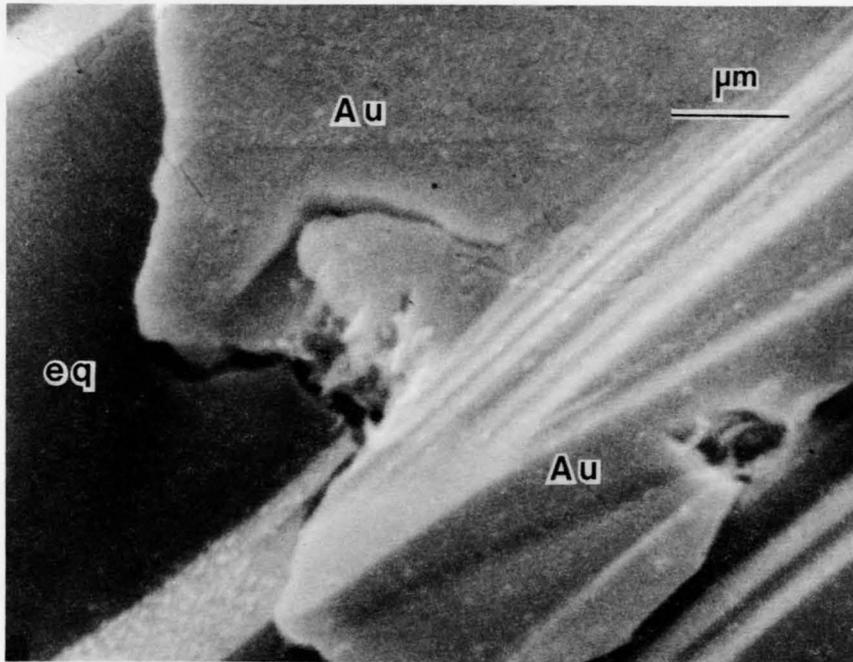
Figure 16. SEM photomicrograph showing gold (Au)- quartz (eq) contact in vein quartz, Parks Mine.
