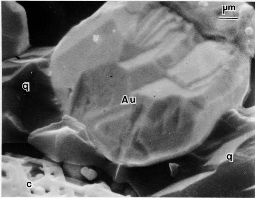
Figure 28. SEM photomicrograph showing euhedral gold (Au) in quartz (q) and near covellite (c), Parks Mine.
