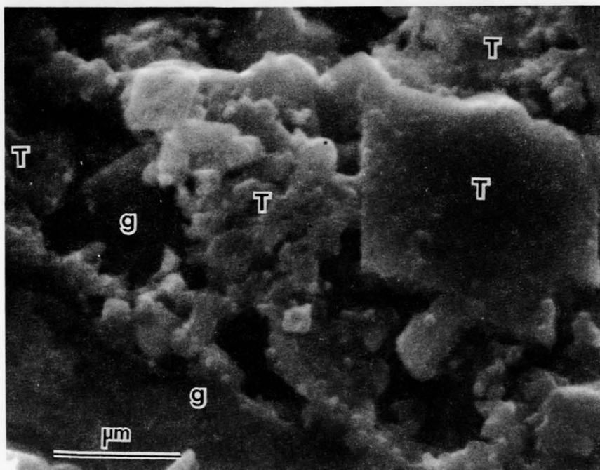
Figure 38. SEM photomicrograph showing some of the better-formed gold-silver telluride (T) associated with altered galena, Parks Mine.
