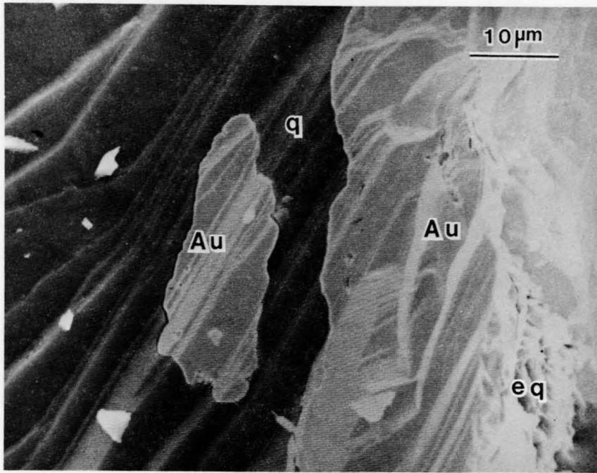
Figure 24. SEM photomicrograph showing magnified view of a portion of Figure 23. Gold (Au), quartz (q), etched-quartz (eq).
