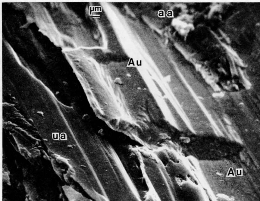
Figure 40. SEM photomicrograph showing gold (Au) deposited along sprung cleavages of amphibole (ua) and replicating both its surface texture and cleavage angles, Latimer Mine. Altered amphibole (aa).
