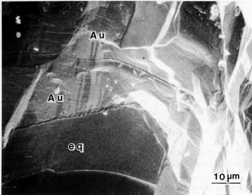
Figure 7. SEM photomicrograph showing gold (Au) enclosing the end of a euhedral quartz crystal (eq), Landers Prospect.
