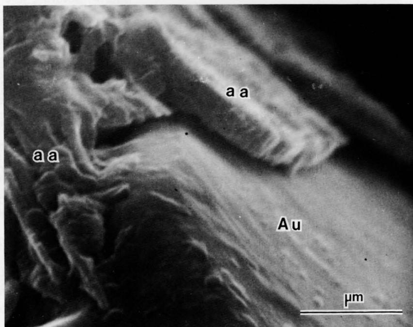
Figure 44. SEM photomicrograph showing uneven surface of gold (Au) which appears to have formed on partly altered amphibole (aa), Latimer Mine.
