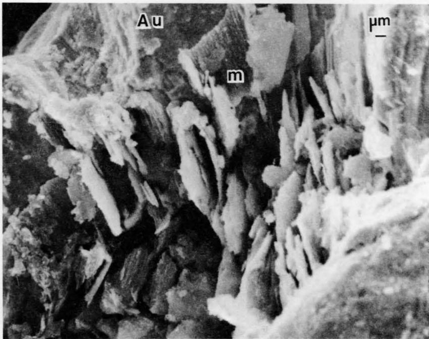
Figure 13. SEM photomicrograph showing a replicating gold (Au) particle in which the ends of some mica (m) books still are embedded, Landers Prospect.
