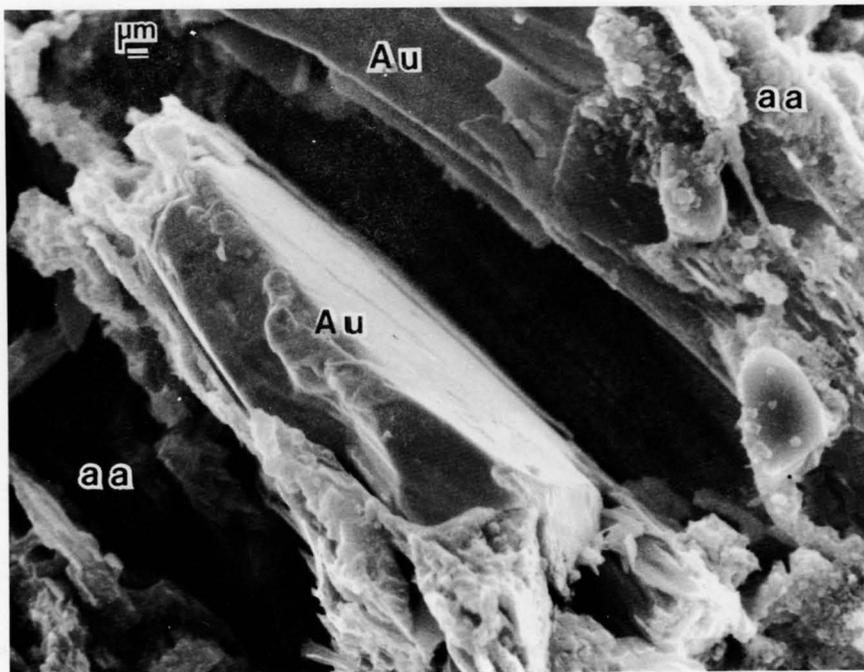
Figure 42. SEM photomicrograph showing gold (Au) in amphibole (aa) partly altered to limonite, Latimer Mine.
