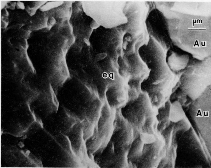
Figure 18. SEM photomicrograph showing etched quartz (eq) surface over which gold (Au) was deposited, Parks Mine.
