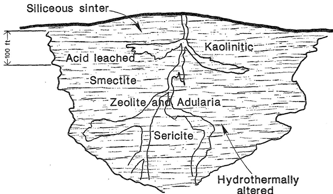
Figure 47. Alteration model of a typical hot spring system.
