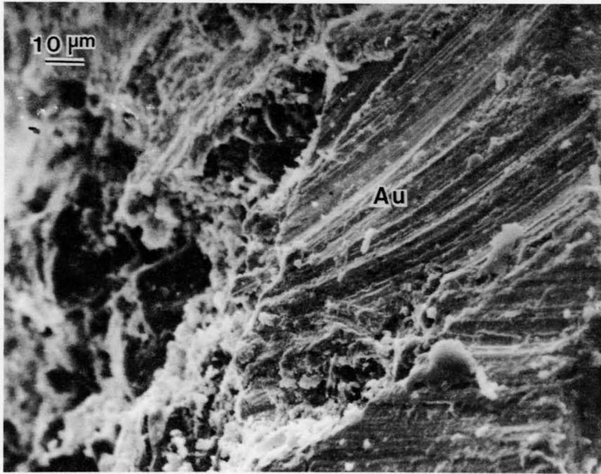
Figure 12. SEM photomicrograph showing gold (Au) surface which is a cast of the mica books against which it was deposited, Landers Prospect.
