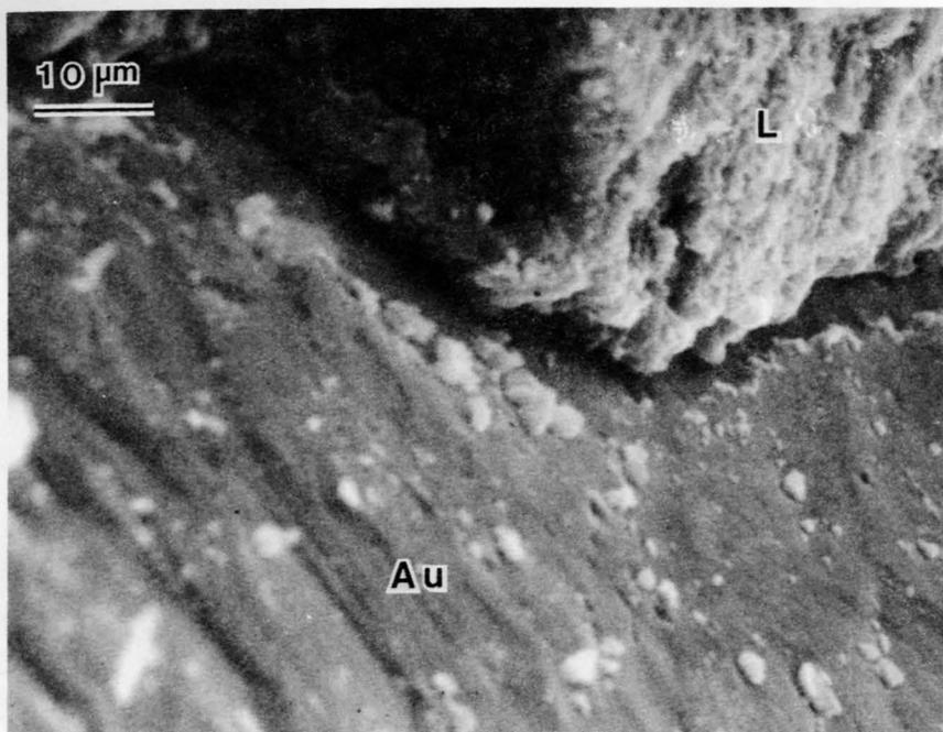
Figure 11. SEM photomicrograph showing gold (Au) particle against pyrite replicating its striated and perhaps slightly altered surface, Landers Prospect. Afterward, the pyrite was altered almost completely to porous limonite (L).
