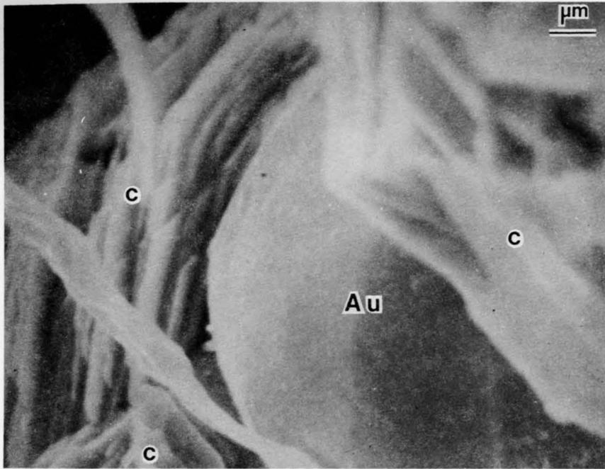
Figure 30. SEM photomicrograph showing subhedral gold (Au) associated with covellite (c), Parks Mine.
