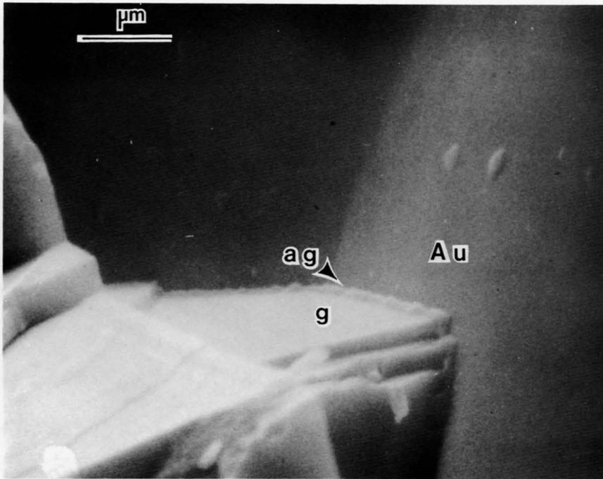
Figure 35. SEM photomicrograph showing the planar gold (Au)-galena (g) contact in Figure 34. Altered galena (ag).
