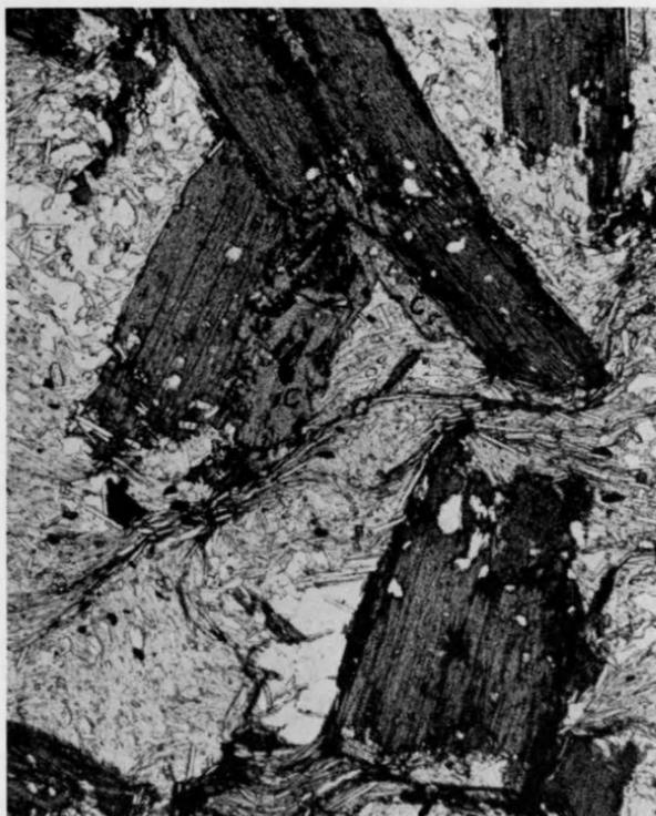
Fig 18. Microphotograph, plain light, S29. X-biotite schist. Dark biotite porphyroblasts in a fine quartz-sericite matrix. The biotite has partly altered to chlorite (c) which is dusted by opaque matter.
