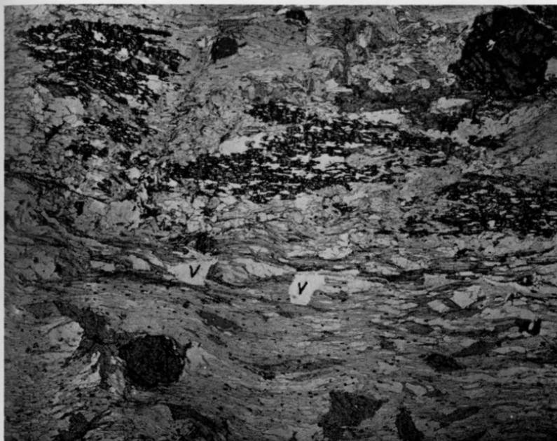
Fig. 9. Microphotograph, plain light. X7. Staurolite and garnet porphyroblasts in a matrix of biotite (dark gray), muscovite (lighter gray), and quartz (lightest gray); voids are marked by a V.
