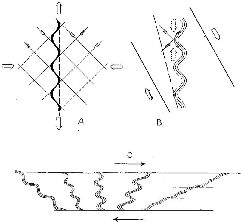
Fig. 51. A. Crinkling by simultaneous shear along two sets of planes. B. Crinkling by flexure of earlier planes. Large open arrows indicate componental movements, single-barbed arrows show relative movement in a smaller domain. C. Ideal configuration of homogeneous planes externally rotated by crinkling; successive stages left to right. Compare with Plate 6. Variation in the configuration of the crinkles is evidence of inhomogeneous deformation.
