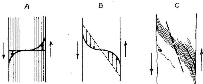
Fig. 48. A. Passive bending of a mechanically unimportant plane. B. Flexure of a mechanically effective plane. C. Flexure of cleavage in mica schist. The dashed line indicates the initial orientation of the deformed plane.
