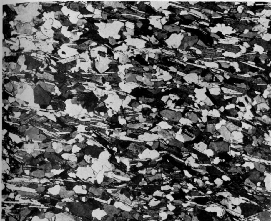
Fig. 5. Microphotograph, crossed nicols, X26. Metagraywacke, composed of quartz, oligoclase, biotite, muscovite, and accessory minerals. (Original grain shapes are visible only with uncrossed nicols.)
