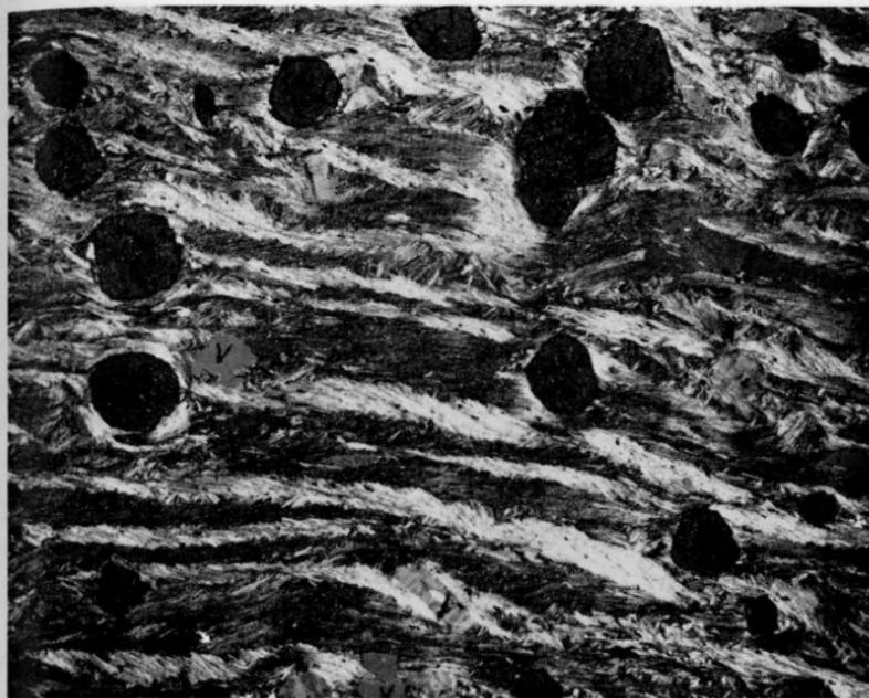
Fig. 8. Microphotograph, nicols partially crossed, X7. Garnet-mica schist. The voids are marked by a V. The other large, clear areas are andesine grains.
