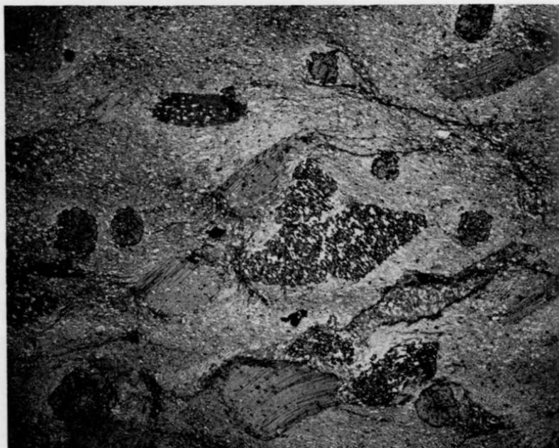
Fig. 10. Microphotograph, plain light X7. Staurolite, garnet, and biotite porphyroblasts in a fine matrix of muscovite and quartz.
