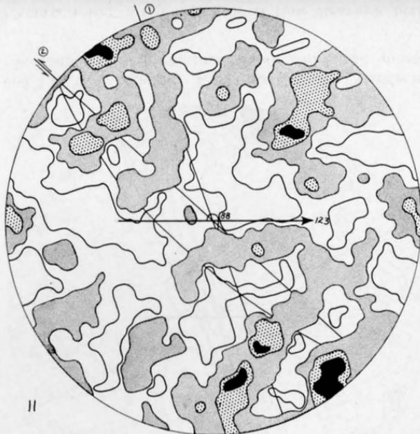
Diagram No. 11. Same slide as No. 10. 164 axes of large quartz grains. 3-2-1-0 (max. 3.5%). ① and ② same as No. 10.
