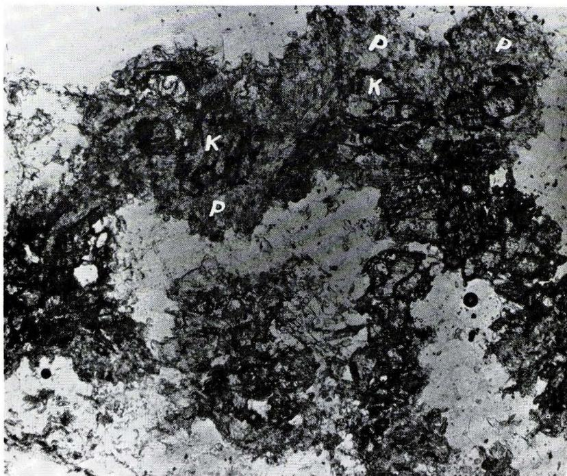
Figure 16—Advanced stage of marginal alteration of kyanite (k) to pyrophyllite (p). Plain light,  $\times 55$ .
