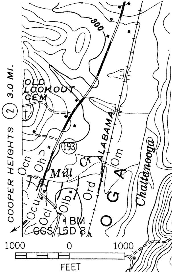
Figure 4—Geologic contacts at the Mill Creek Section, Chattanooga Valley, Kensington quadrangle (fig. 1, Map Number—2). Murfreesboro Limestone—Om; Ridley Limestone—Ord; Lebanon Limestone—Oib; Carters Limestone, lower member—Ocl, upper member—Ocu; Hermitage Formation—Oh; Cannon Limestone—Ocn. Base from USGS-TVA Kensington Quadrangle; contour interval 20 feet.
