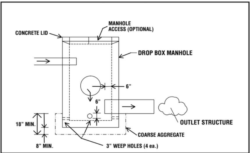
Example of typical drop inlet box diagram.
