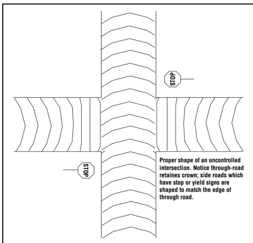
Illustration of proper crown shape at controlled intersections. Curved lines indicate road crowns at intersection.
