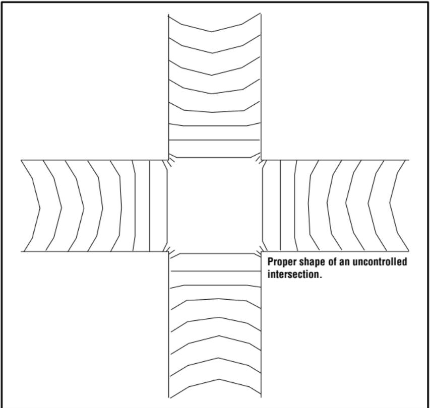
Proper crown shape at uncontrolled intersections.
