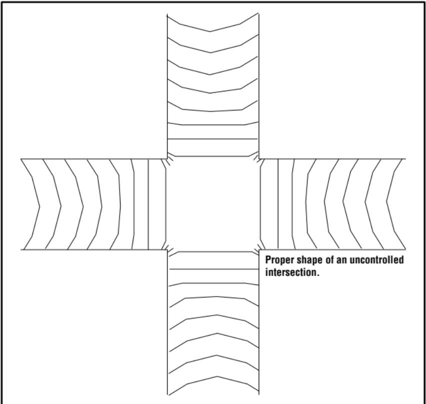
Proper crown shape at uncontrolled intersections.
