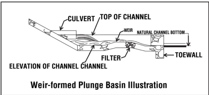
Typical layout of plunge pool to reduce water energy.
