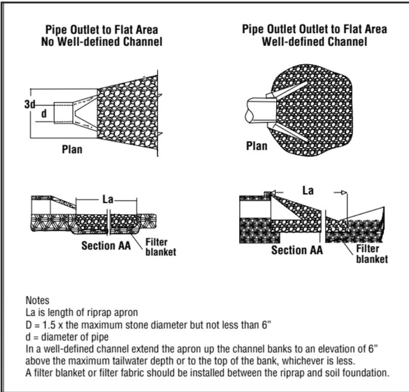
Typical storm drain (St) outlet protection apron.
