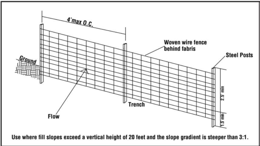
Illustration of Type C silt fence.
