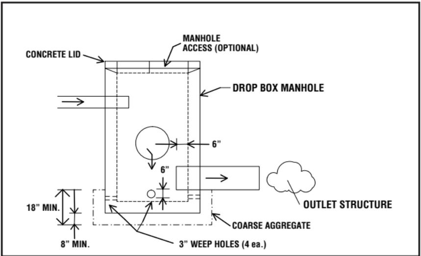
Example of typical drop inlet box diagram.
