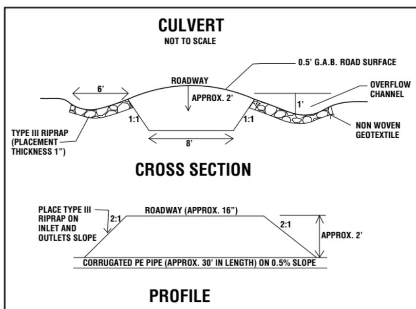
Typical layout profile for culverts and drains.
