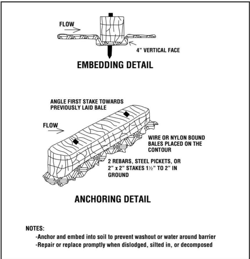
Illustration of bales for temporary erosion control, sediment barrier with hay or straw bales (Sd1-b).
