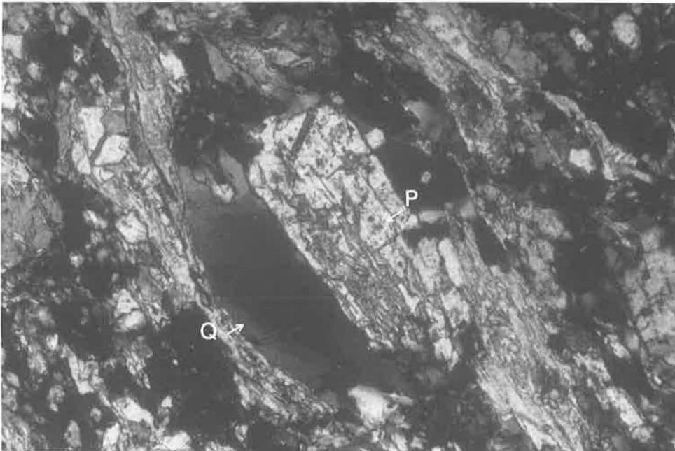
Figure 3. Photomicrograph of a crystal tuff from the northern metavolcanic assemblage. A euhedral plagioclase phenocryst (P) is shown included in quartz (Q). Field of view 1.3mm.
