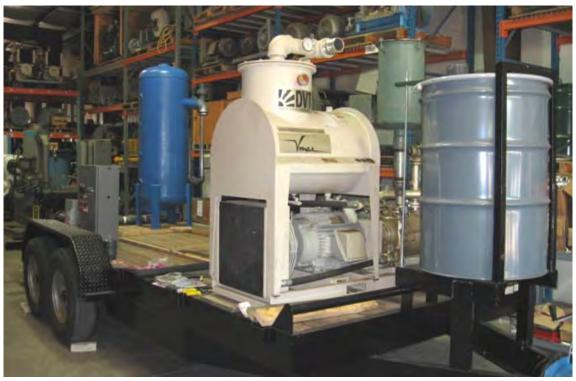
Portable multi-phase extraction system – front view. The air/water separator is the blue tank at the rear. The liquid ring vacuum pump is the cream-colored device in the foreground. The granular activated carbon (GAC) air treatment tank is the 85-gallon drum on the right.
