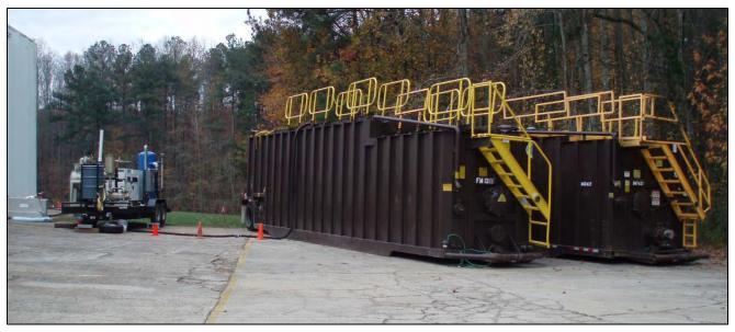
The portable MPE system (left) with the water untreated water discharge line running to the on-Site holding tanks (right).
