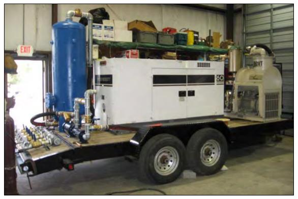
Portable multi-phase extraction system – side view. The air/water separator is the blue tank on the left. The liquid ring vacuum pump is the cream-colored device on the right. The diesel power generator is in the middle.
