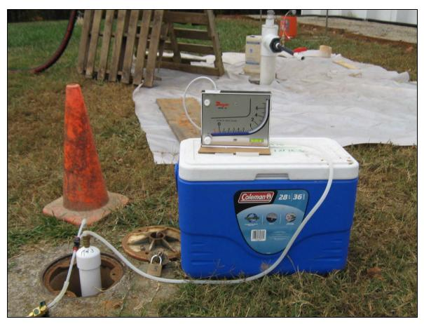
Typical outdoor monitoring well instrumented with a vacuum gauge (sitting on top of the cooler). Extraction well MP-2 is in the background.
