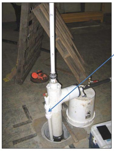
Typical setup of the slurp tube inserted into the wellhead during operation (MP-1 shown). Various valves and gauges allow for the control and monitoring of the applied vacuum at the wellhead. The collocated piezometer next to the larger extraction well is shown.
