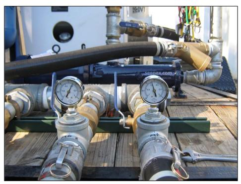
Intake manifold with vacuum gauges mounted at the rear of the trailer.
