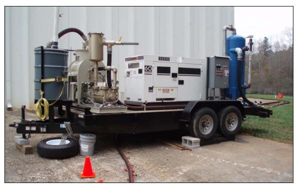
Portable multi-phase extraction system setup at the Site.
