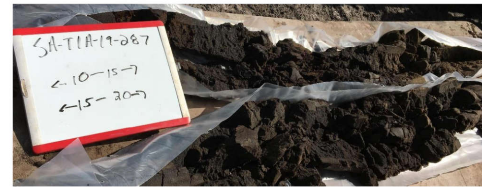
PHOTOGRAPH 3. UNCONSOLIDATED BLACK SAND
