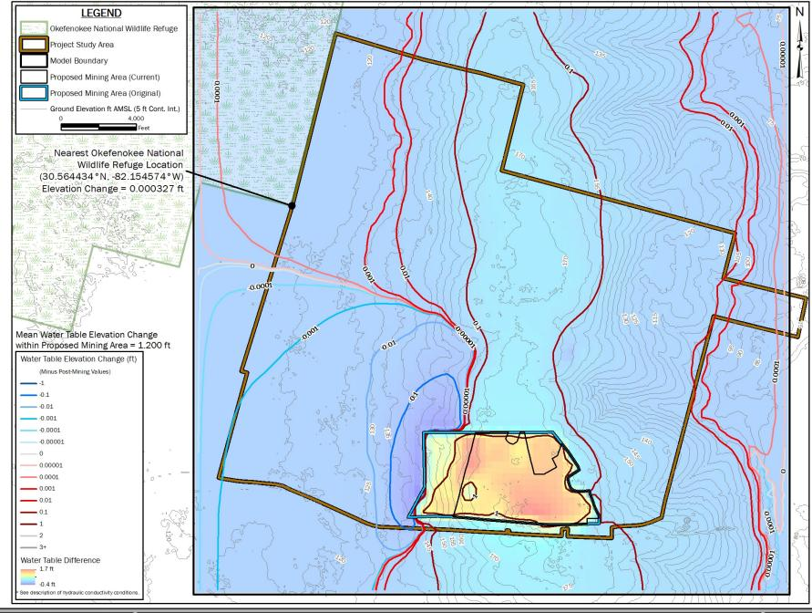
FIGURE 12: HYDRAULIC HEAD DIFFERENCE BETWEEN HOMOGENEOUS SCENARIO MODELED HERE & POST-MINING SCENARIO OF HOLT ET AL. (2020); THE VERTICAL & HORIZONTAL K OF THE UPPER 10 FEET OF THE MINE FOOTPRINT IS 1E-06 CM/S
