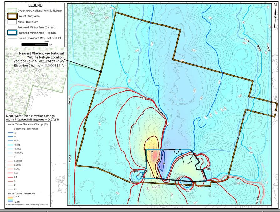
FIGURE 27: HYDRAULIC HEAD DIFFERENCE BETWEEN LAYERED SCENARIO HERE MODELED HERE & PRE-MINING SCENARIO OF HOLT ET AL. (2020); THE VERTICAL EFFECTIVE K OF THE UPPER 10 FEET OF THE MINE FOOTPRINT IS 1E-05 CM/S & THE HORIZONTAL K IS 1E-03 CM/S
