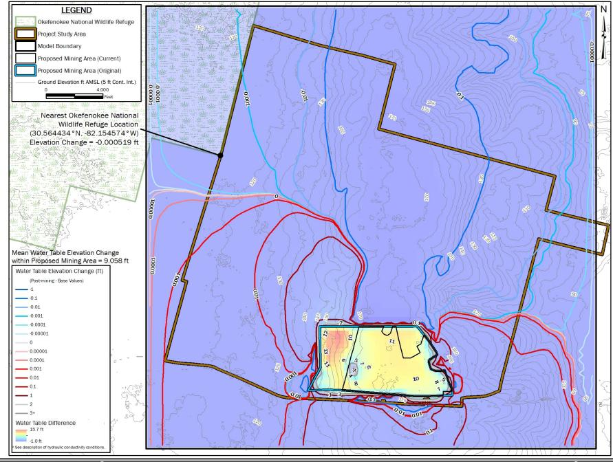
FIGURE 29: HYDRAULIC HEAD DIFFERENCE BETWEEN LAYERED SCENARIO HERE MODELED HERE & PRE-MINING SCENARIO OF HOLT ET AL. (2020); THE VERTICAL EFFECTIVE K OF THE UPPER 10 FEET OF THE MINE FOOTPRINT IS 1E-07 CM/S & THE HORIZONTAL K IS 1E-03 CM/S TWIN PINES MINERALS, LLC SAUNDERS DEMONSTRATION MINE ST. GEORGE, CHARLTON COUNTY, GEORGIA
