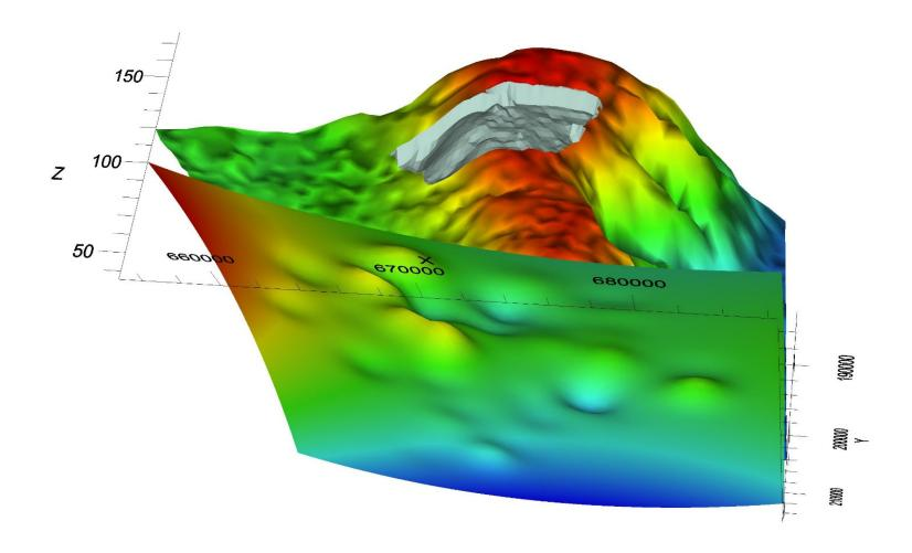
NOTE: Gray area represents the mining area at the top of the Hawthorn layer elevations. The gray area represents the original mine footprint of Holt et al (2020); the current mine footprint does not extend as far west.
