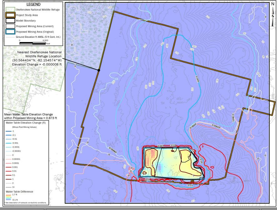
FIGURE 20: HYDRAULIC HEAD DIFFERENCE BETWEEN LAYERED SCENARIO HERE MODELED HERE & POST-MINING SCENARIO OF HOLT ET AL. (2020); THE VERTICAL EFFECTIVE K OF THE UPPER 10 FEET OF THE MINE FOOTPRINT IS 1E-06 CM/S & THE HORIZONTAL K IS 1E-03 CM/S
