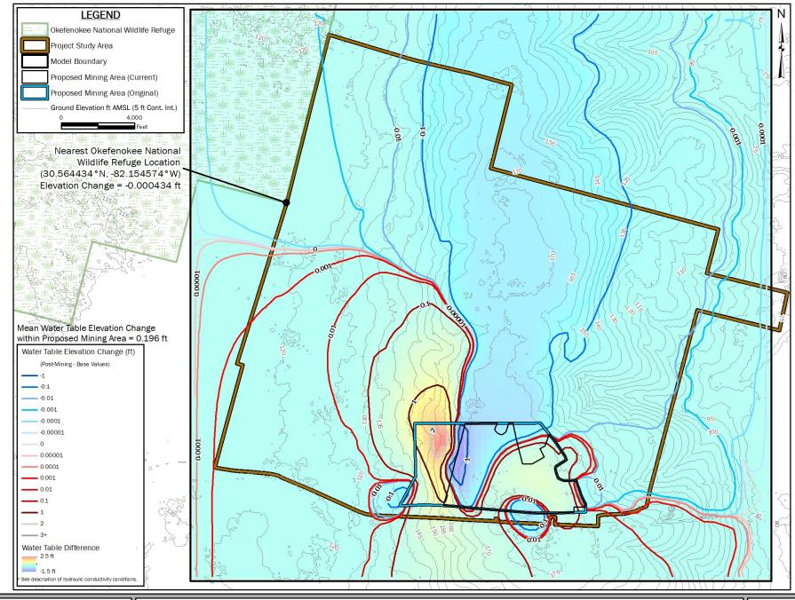
FIGURE 26: HYDRAULIC HEAD DIFFERENCE BETWEEN LAYERED SCENARIO HERE MODELED HERE & PRE-MINING SCENARIO OF HOLT ET AL. (2020); THE VERTICAL EFFECTIVE K OF THE UPPER 10 FEET OF THE MINE FOOTPRINT IS 1E-04 CM/S & THE HORIZONTAL K IS 1E-03 CM/S TWIN PINES MINERALS, LLC SAUNDERS DEMONSTRATION MINE ST. GEORGE, CHARLTON COUNTY, GEORGIA
