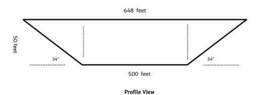
Figure 2. Mine Pit Conceptual Model (X-section and Profile)
