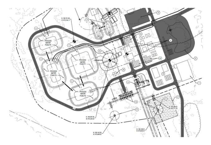
The Process Water Ponds (P1–P4) will be above-ground and lined. Lining details for all ponds are shown on Sheet C-701. The individual pond volumes are shown on Sheet C-200; as shown in the table below, the total capacity of the four ponds is approximately 3.9 MG, and the working capacity with appropriate freeboard is 3.4 MG.
