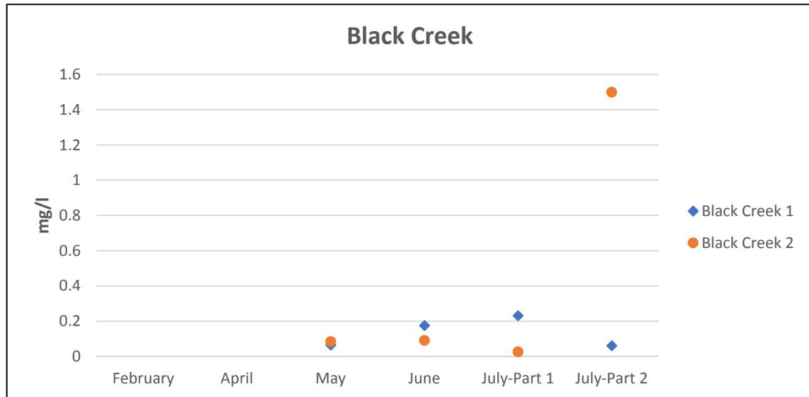
Figure 3.8: Ammonia as N concentration in (a) Iric Branch, (b) Ash Branch, (c) Mill Creek, and (d) Black Creek
