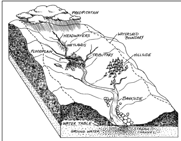
Figure 1.1: Cross section of a watershed.
