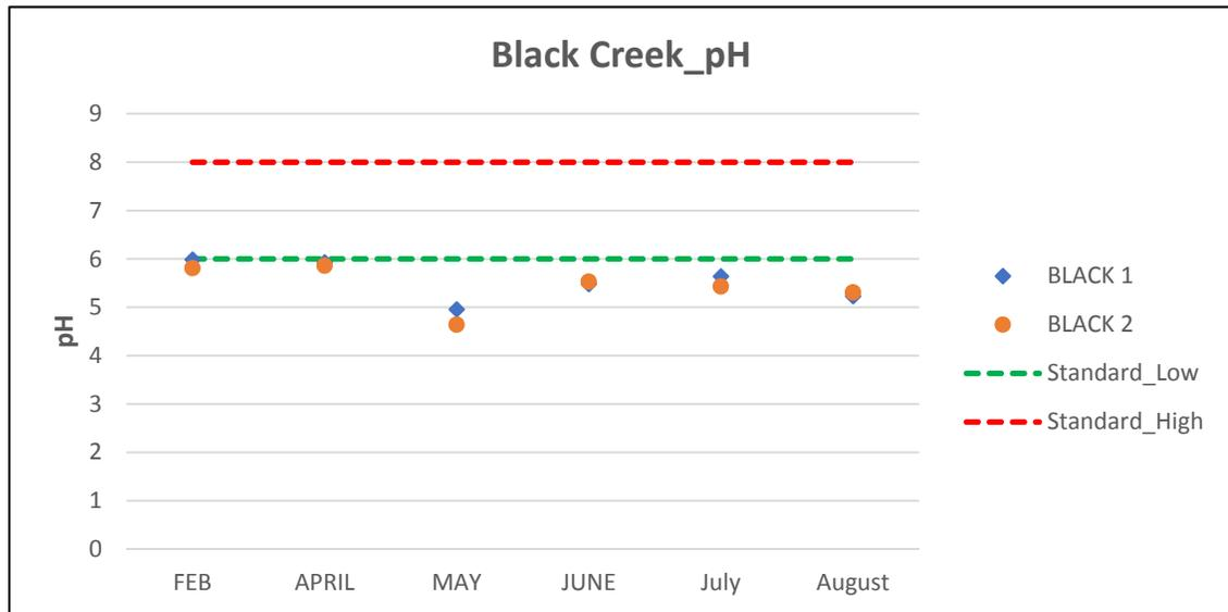
Figure 3.9: pH concentration in (a) Iric Branch, (b) Ash Branch, (c) Mill Creek, and (d) Black Creek
