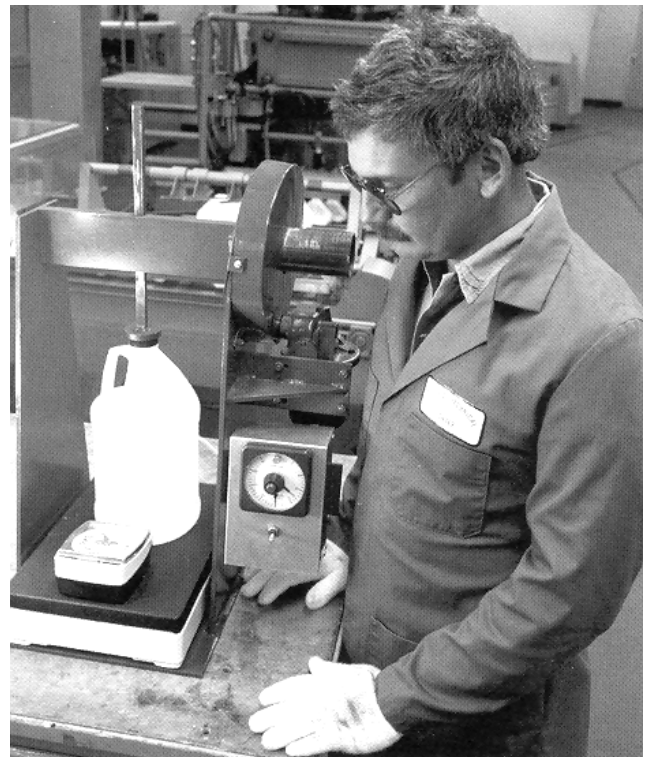
Top-load testing of Marlex ® HDPE containers
