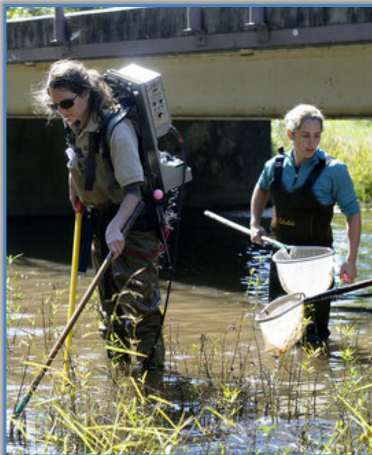
Figure 3.2.a. Sampling with backpack electrofishing equipment.
