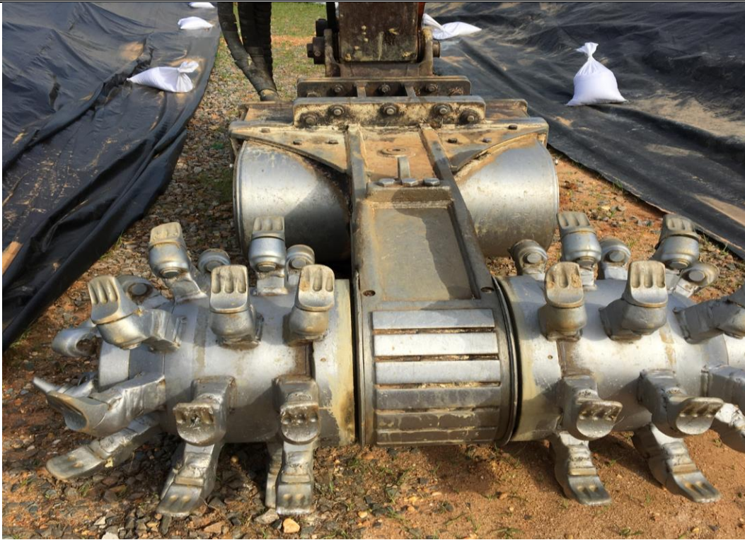
View of soil mixing attachment.
