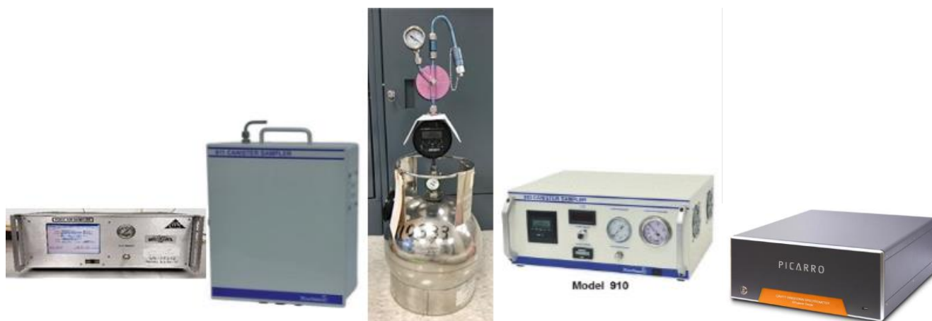
Figure 15. Samplers Used to Collect Ethylene Oxide Data in Georgia (from left to right: ATEC 2200, Xonteck 911, Entech CS1200E passive sampler, Xonteck 910, Picarro G2920)
