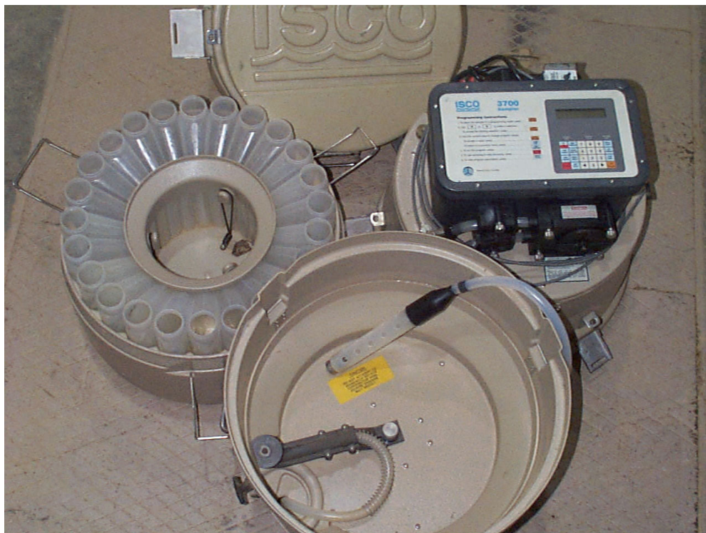
Figure 2- 5 ISCO sampler components clockwise from top: lid, computer and power module, sample distribution arm and pick-up tube, base with 24 1-liter bottles.
