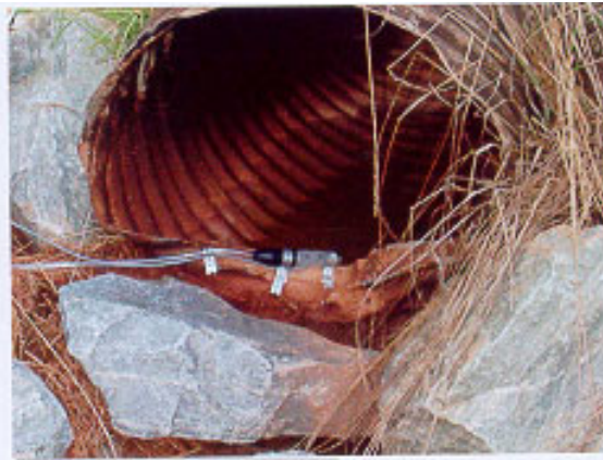
Figure 4-3. 3 Basin discharge point with sampler.
