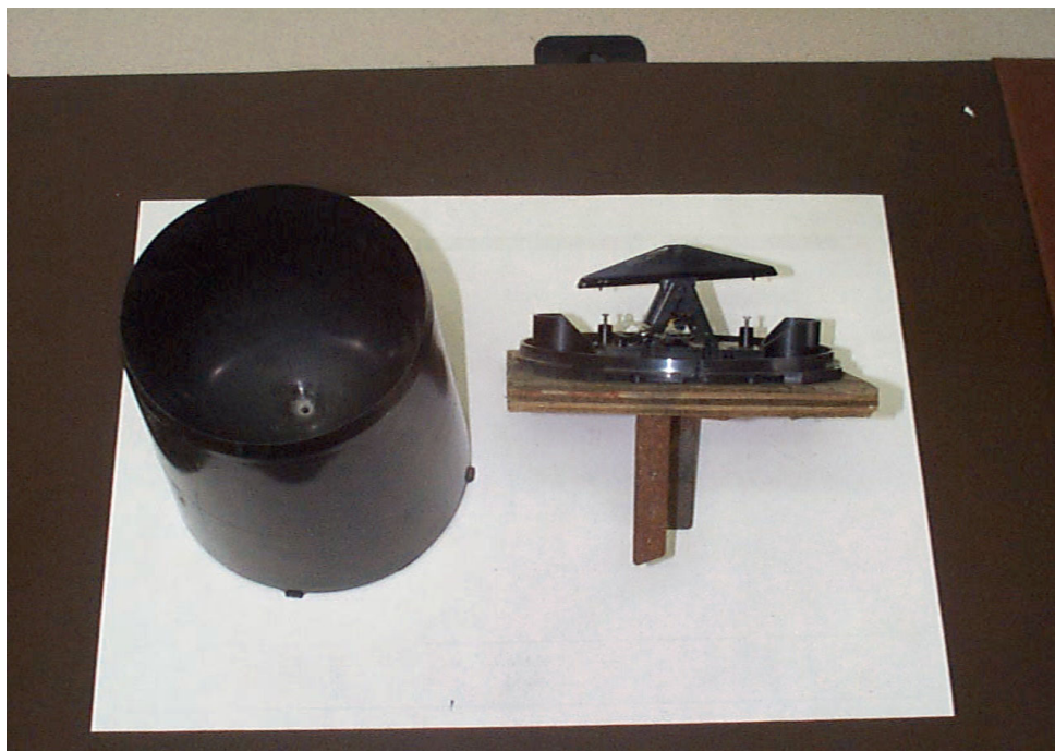
Figure 2- 1 Rain collector showing collection cone and internal tipping bucket.
