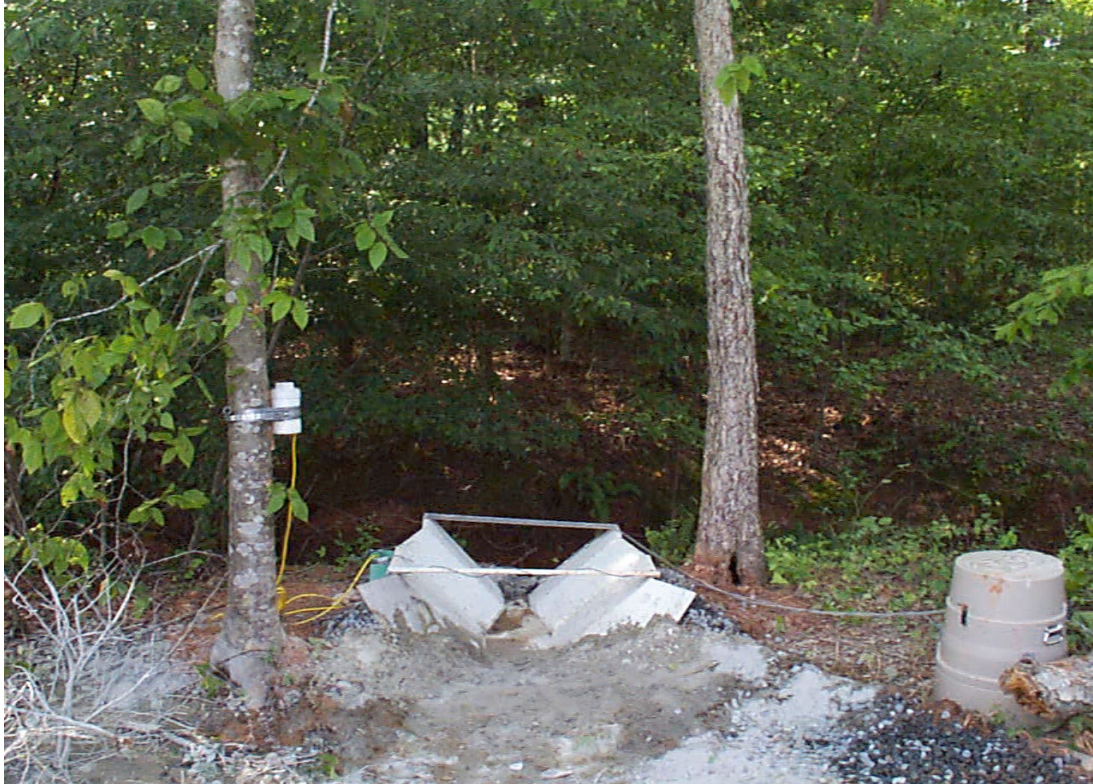
Figure 2- 3 Trapezoidal flume installed at site 1 with stilling well in green on left and ISCO sampler on right.
