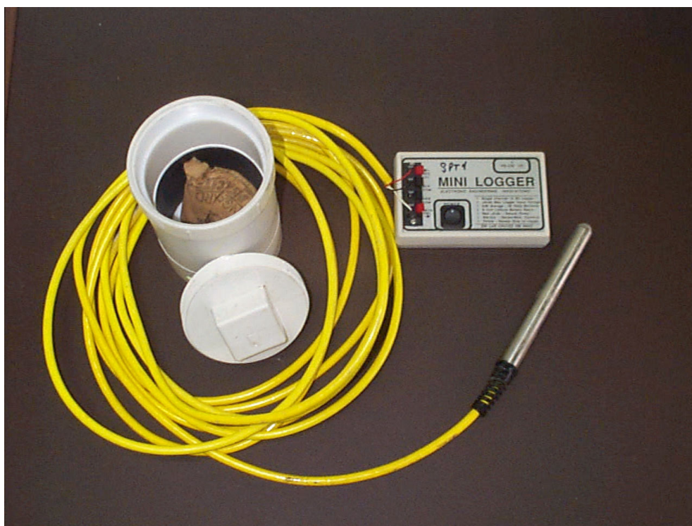
Figure 2- 2 Pressure sensor and data logger assembly for continuous stage recording.
