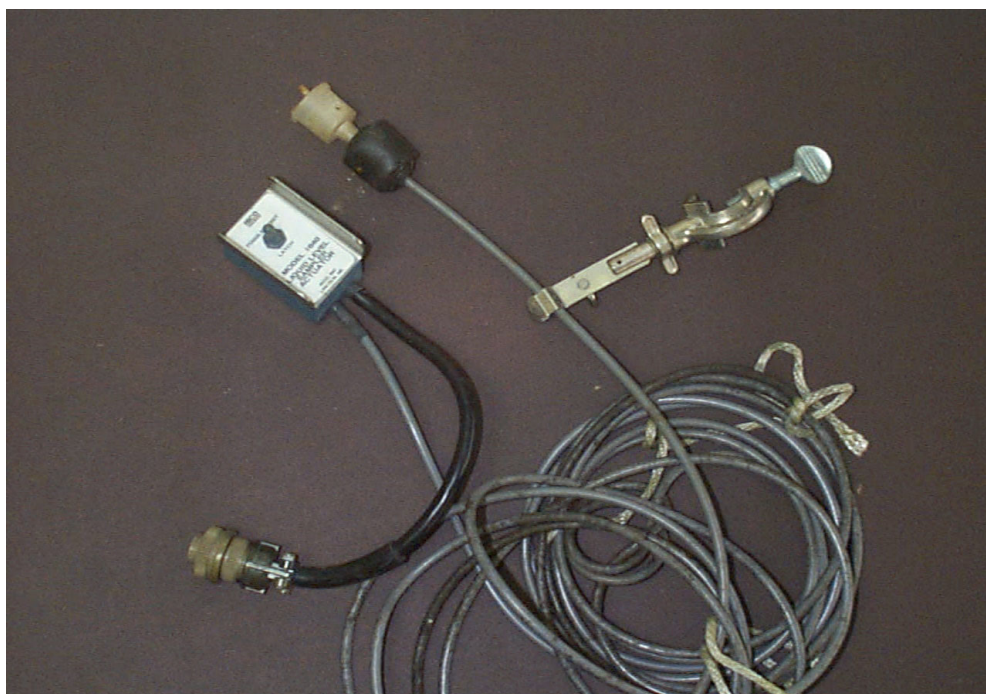
Figure 2- 6 Liquid level actuator showing sensor probe, control box, and related cables.
