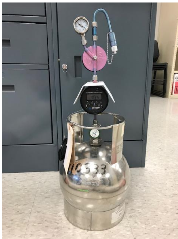
Figure 17. Entech CS1200E Passive VOCs Sampler Set-Up
