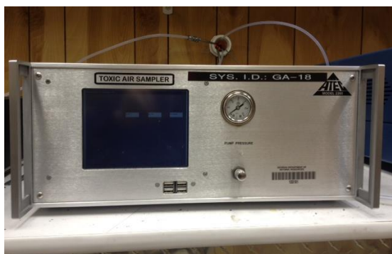
Figure 18. ATEC 2200 VOCs Sampler
