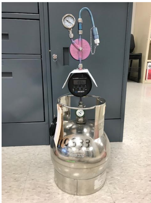
Figure 17. Entech CS1200E Passive VOCs Sampler Set-Up
