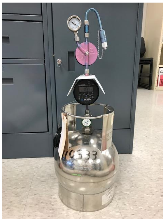
Figure 17. Entech CS1200E Passive VOCs Sampler Set-Up
