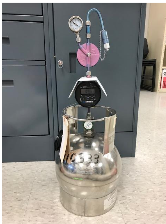
Figure 17. Entech CS1200E Passive VOCs Sampler Set-Up
