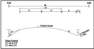
Example of typical road crown profile. Source: Limestone Valley RC&D adapted from GDOT
