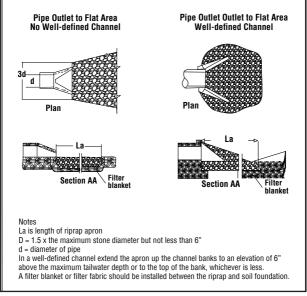
Typical storm drain (St) outlet protection apron. Source: Limestone Valley RC&D adapted from Manual for Erosion and Sediment Control in Georgia, GSWCC
