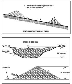
General spacing and layout of rock check dams (Cd). Source: Limestone Valley RC&D Council adapted from Manual for Erosion and Sediment Control in Georgia, GSWCC
