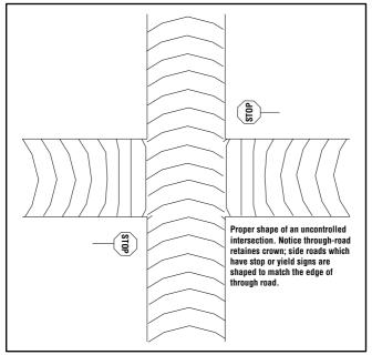
Illustration of proper crown shape at controlled intersections. Curved lines indicate road crowns at intersection. Source: Limestone Valley RC&D adapted from Federal Highway Administration, South Dakota LTAP Manual
