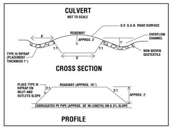
Typical layout profile for culverts and drains. Source: Limestone Valley RC&D adapted from Manual for Erosion and Sediment Control in Georgia, GSWCC
