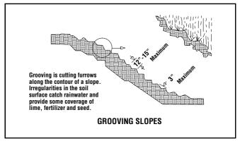
Typical serrated (grooved) slope stabilization layout, a surface roughening (Su) practice.
