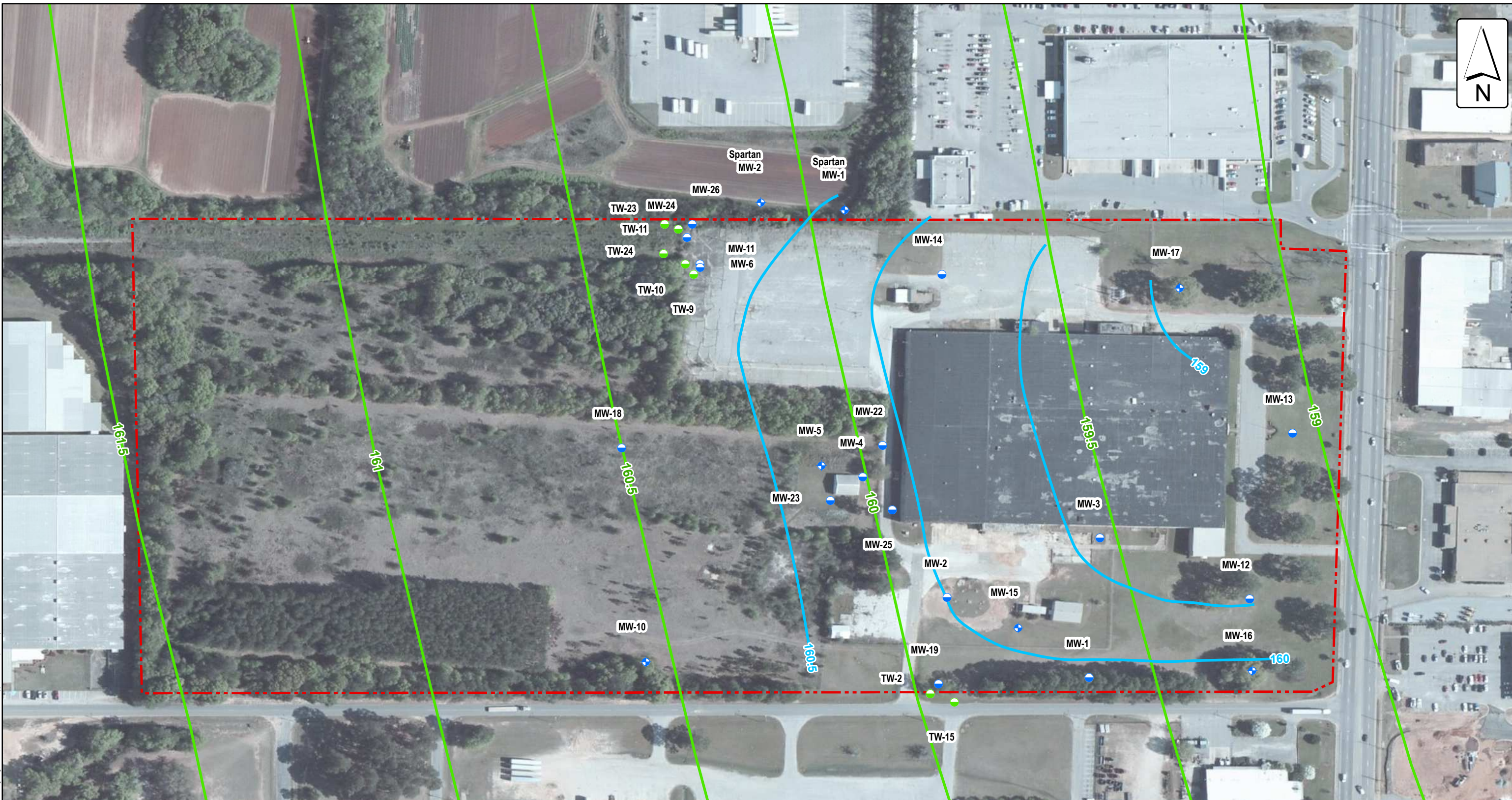
Figure 9 Modeled Heads Versus Lower Water Bearing Zone Potentiometric Surface Map March 2014
