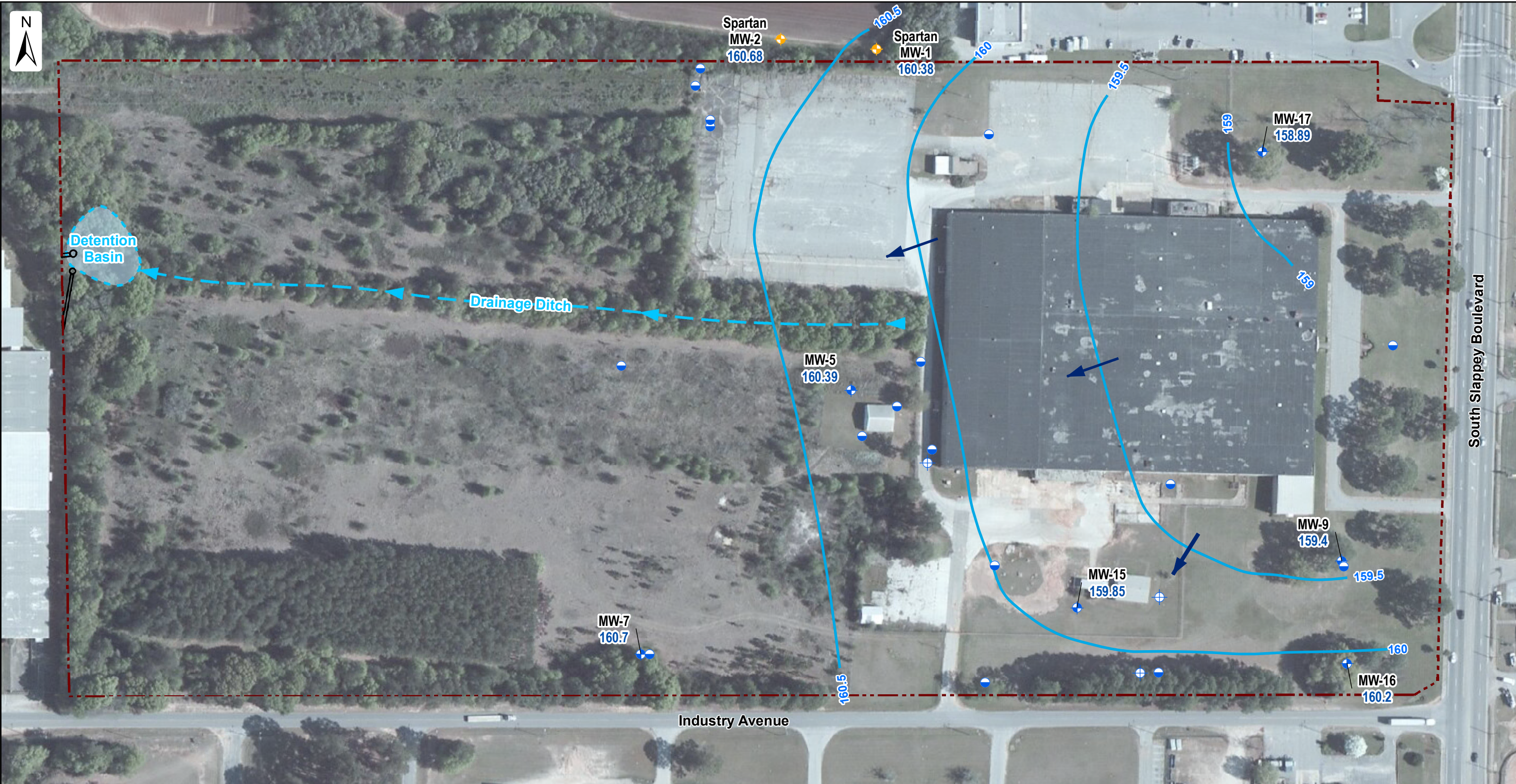
Figure 6 Potentiometric Surface Map Lower Water Bearing Zone March 26, 2014
