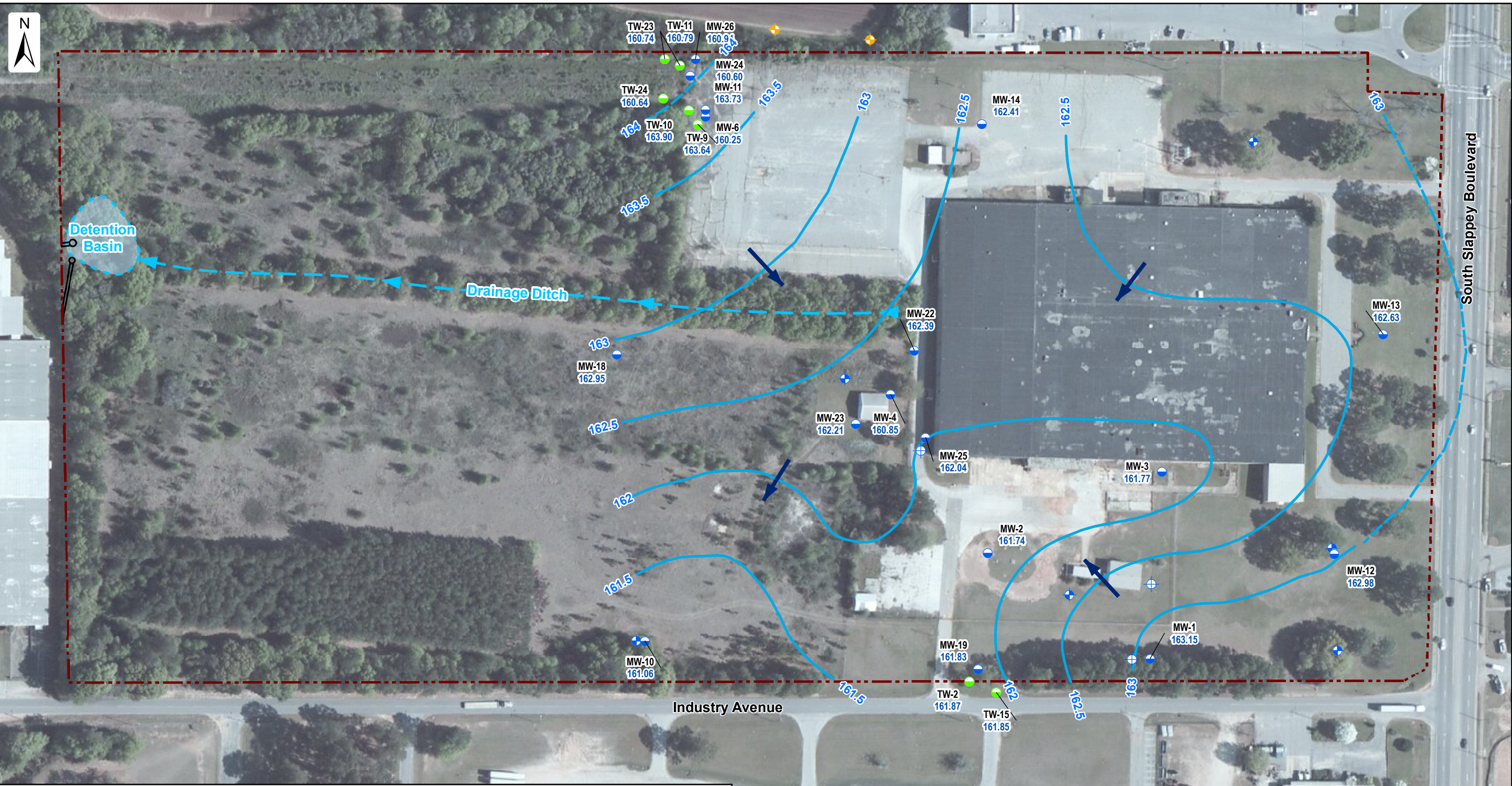
Figure 5 Potentiometric Surface Map Upper Water Bearing Zone March 26, 2014
