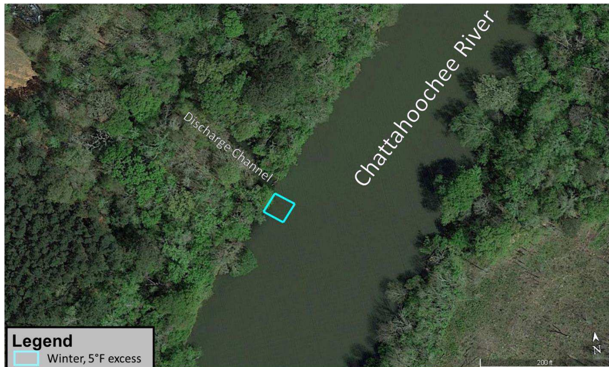
Figure 6: Mixing zone during critical conditions for the 5°F excess temperature (winter) temperatures
