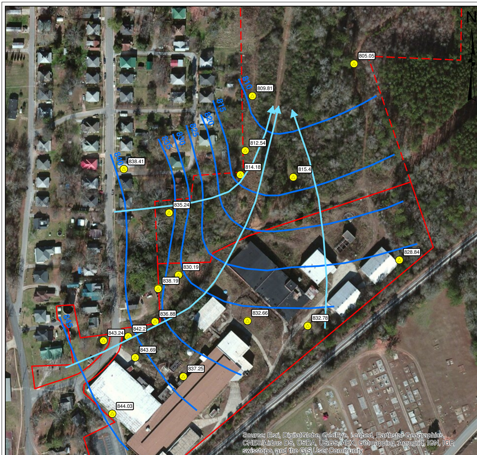
Figure 5 Site Potentiometric Surface and Groundwater Flow Direction Grantville Mill Grantville, Georgia
