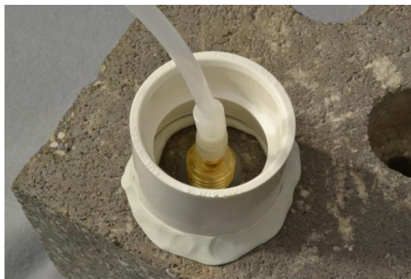
Figure 6. Water dam used for leak detection
