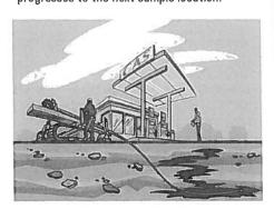
The soil samples collected using these techniques are 12 inches in length and slightly less than 2 inches in diameter. Directed
