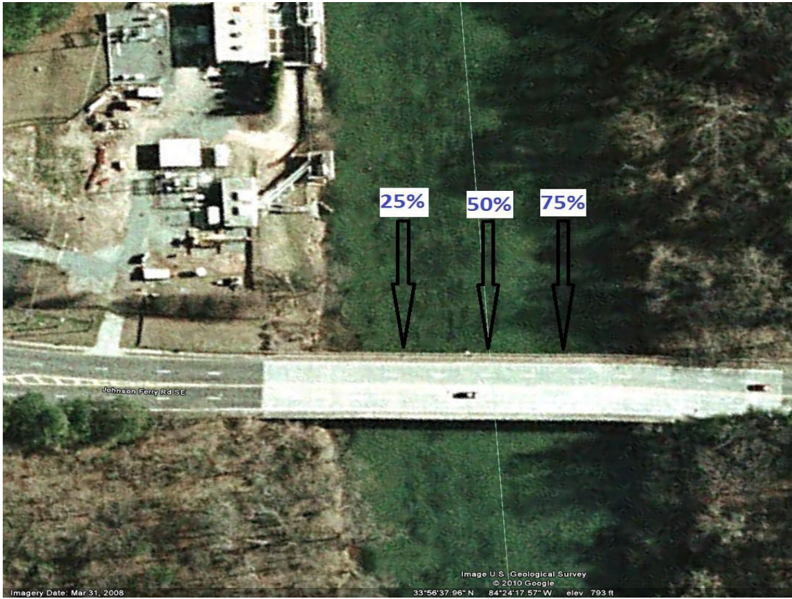
Figure I-1. Three samples are collected across the waterbody: one at the horizontal midpoint of the stream, and one each at points halfway between the midpoint and the edge of downstream flow. Avoid sampling in areas that are stagnant or contain backflow.
