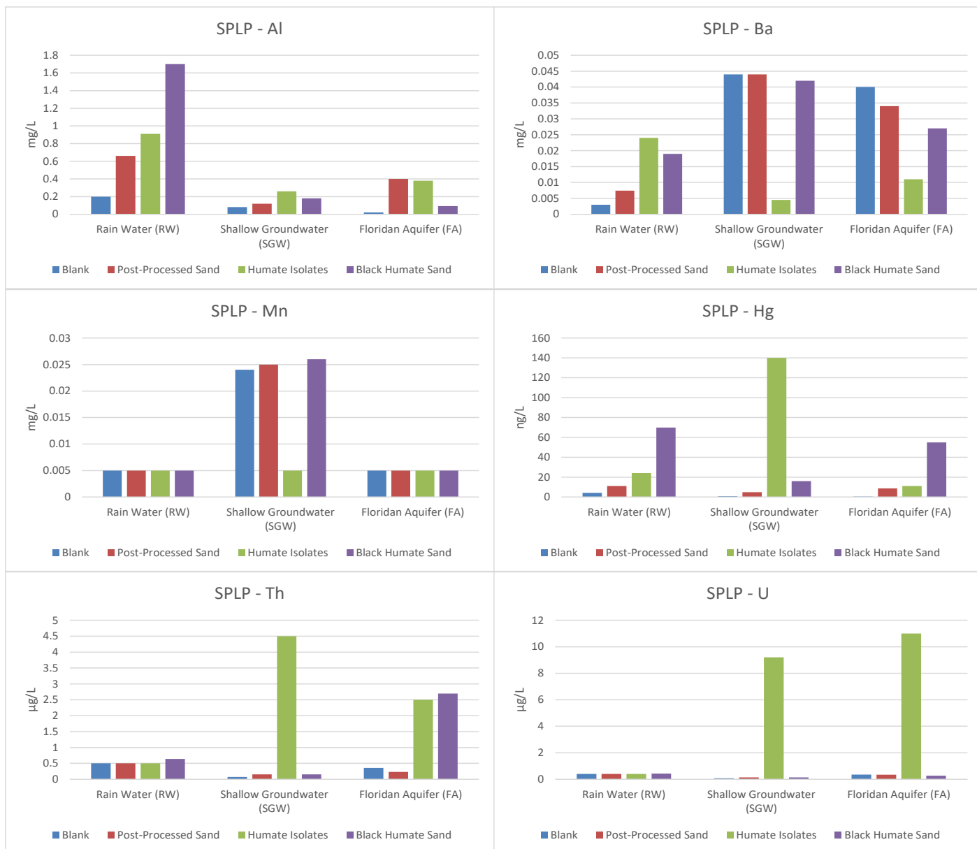
Figure 1. Comparison of SPLP Results Using Rainwater, Local Shallow Groundwater, and Floridan Aquifer Water July 2021 Addendum to the November 2020 Geochemical Testing and Evaluation Memorandum
