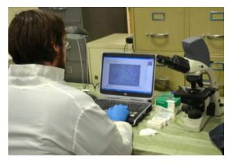
A Digital Microscope is connected to a laptop computer with proprietary "Droplet Size Calculation Software"
