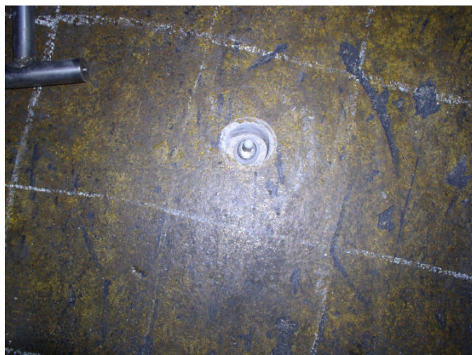
Vapor Pin™ sub-slab sampling point
