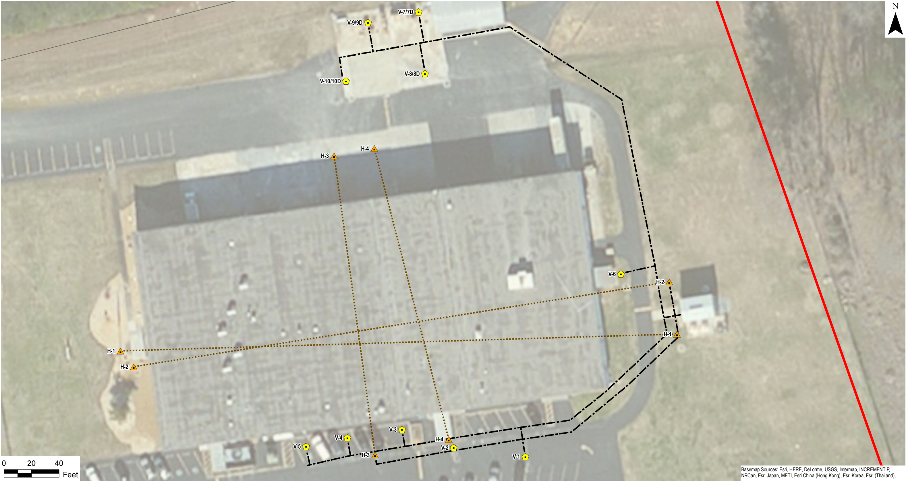
FIGURE 2-2 - SOIL VAPOR EXTRACTION SYSTEM VIRP Report Murata Erie N.A., Inc. Rockmart, Georgia
