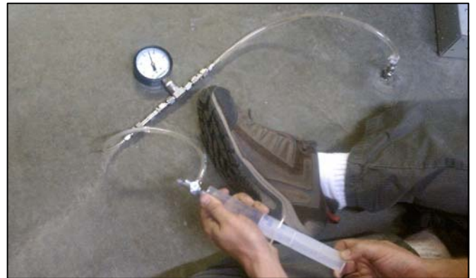
Photo 10 - Purging sample tubing prior to vapor sampling, BV051211-001; May 12, 2011
