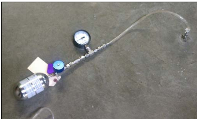
Photo 11 - Sub-slab vapor sampling with 400-ml mini-can, BV051211-001; May 12, 2011
