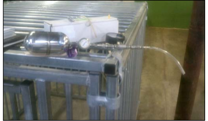
Photo 14 - Blank sampling (ambient air, equipment blank); May 12, 2011
