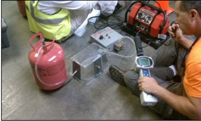
Photo 13 - Shroud leak testing at BV051211-003; May 12, 2011
