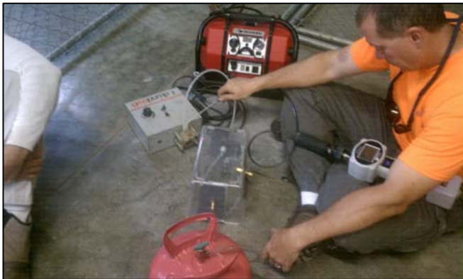
Photo 9 - Shroud leak testing at BV051211-001; May 12, 2011
