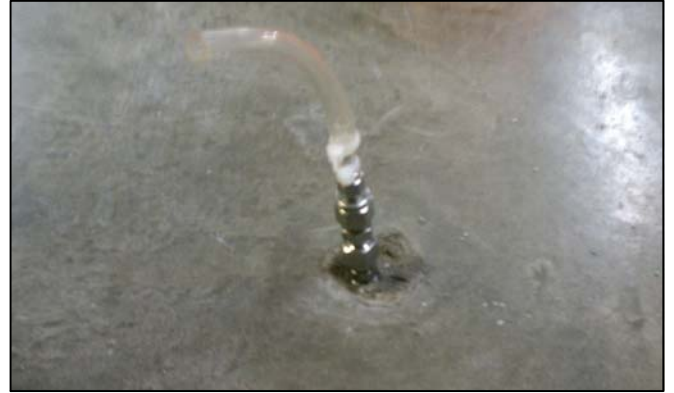
Photo 8 - Implant sampling set-up, BV051211-001; May 12, 2011
