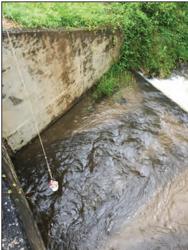
A weighted sampling yoke was used to collect samples from bridges and roadways.
