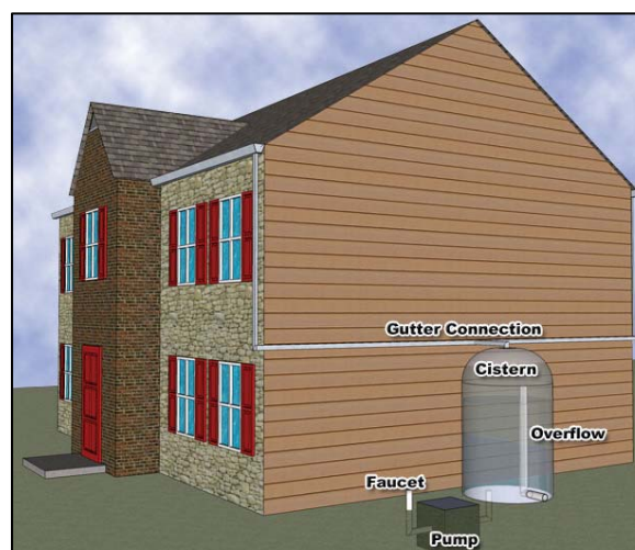
Figure 7.42: Major Components of a Rainwater Harvesting System
