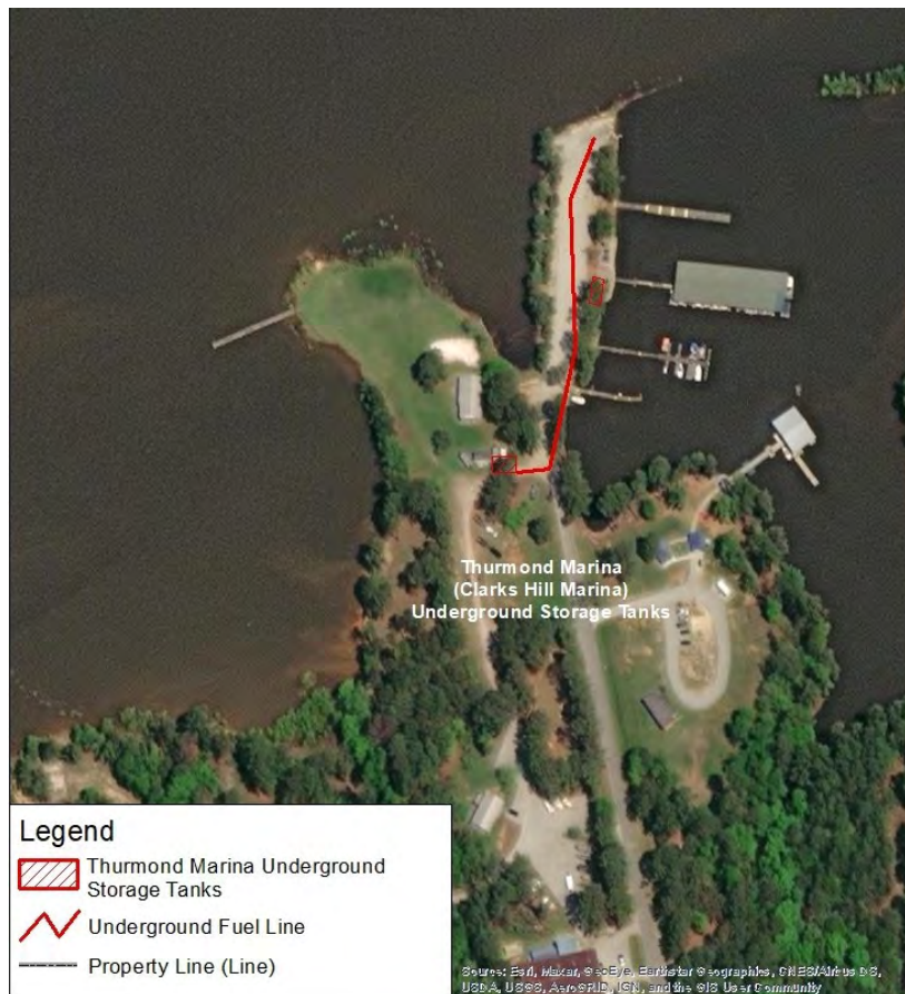
Figure 4: Clarks Hill Marina Underground Storage Tanks and Fuel Line
