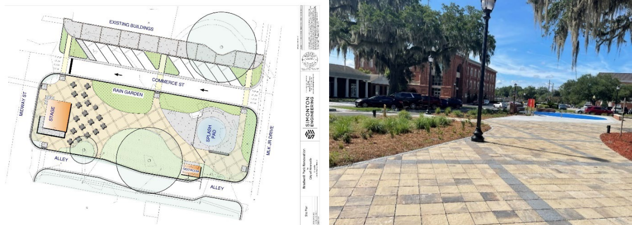
Figure 4: Bio-infiltration BMPs in Bradwell Park - FY2019 Peacock Creek Restoration: Green Infrastructure Demonstration in Downtown Hinesville, Georgia
