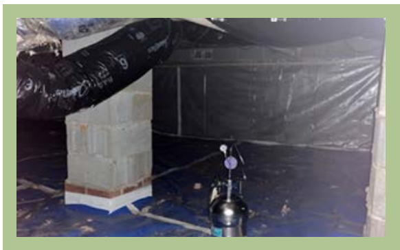
Canister for collecting indoor air readings in crawl space
