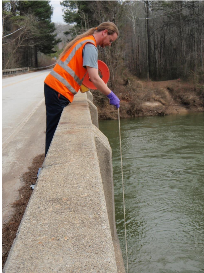
Figure I-2. Take care to minimize rope contact with the side of the bridge when collecting samples.
