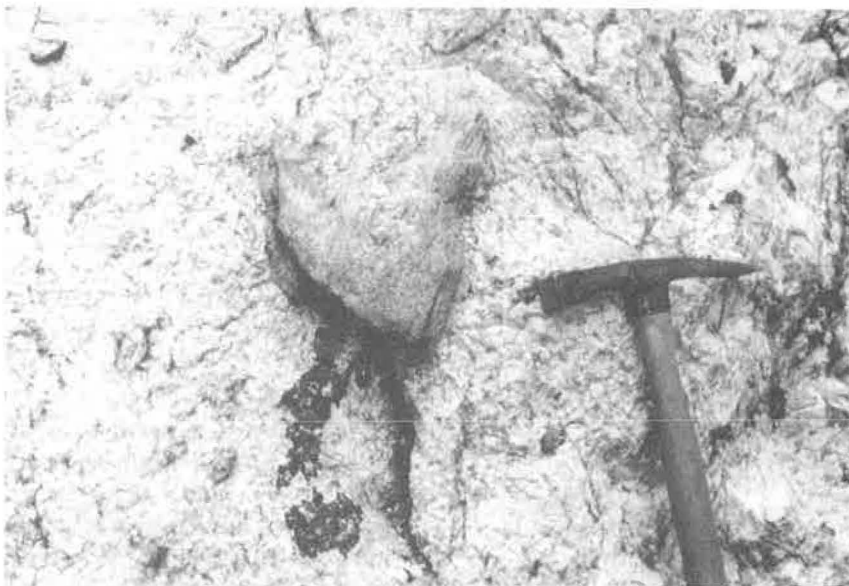
Figure 20. Inclusions of mica schist in the Marblehill pegmatite. Tourmaline forms within the pegmatite in close proximity to the inclusions. The schist may have provided a source for boron by pegmatite-wall rock reactions.
