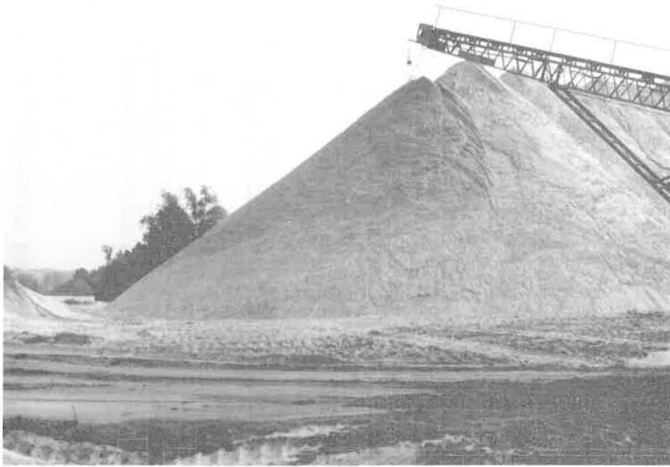
Figure 128. Stock piles of Mortar and Concrete Sand at Satilla Sand Company, Long County.
