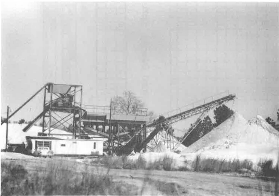
Figure 69. View of classifiers and conveyor belt at Coastal Sand Company, Eden, Georgia.
