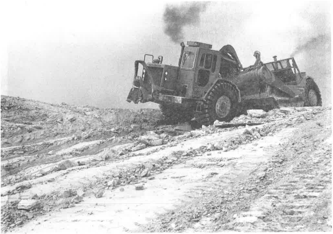
Fig. 1 . Twin engine motor scraper mining kaolin.
