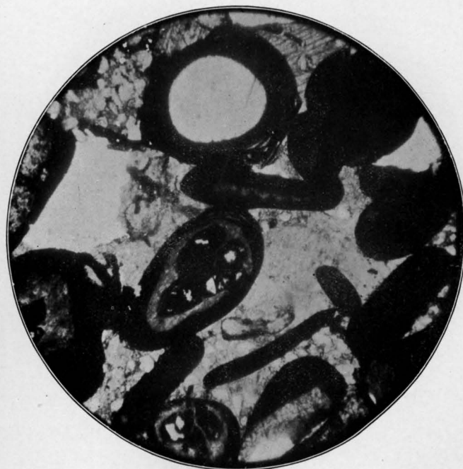
FIG. 2 PHOTO-MICRHGRAPH SHOWING IRON OXIDE GRANULES HAVING A CONCRETIONARY STRUC- TURE IN A MATRIX OF CALCITE. Magnified 75 Diameters.
