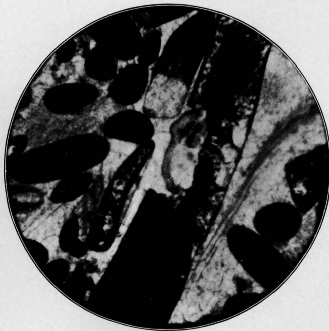
FIG. 2. PHOTO-MICROGRAPH SHOWING NEAR THE CENTER A LONG FRAGMENT OF SHELL WITH ONE END COMPLETELY REPLACED BY IRON OXIDE AND THE OTHER CONSISTING CHIEFLY OF UNALTERED GLAUCONITE. Magnified 75 Diameters.
