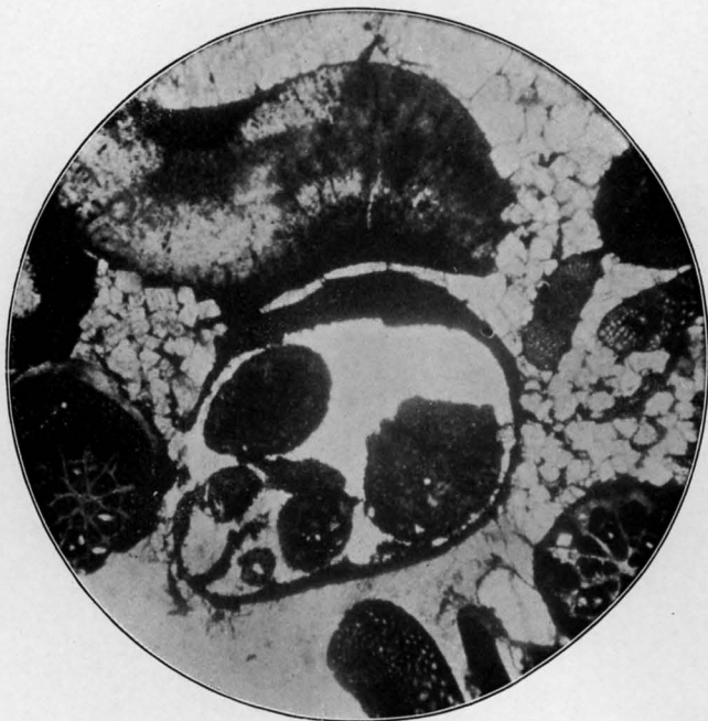
FIG. 1. PHOTO-MICROGOAPH SHOWING NEST OF IRON OXIDE SPHERULES AND FRAGMENTS OF FOSSILS IN GROUND MASS OF CALCITE. Magnified 75 Diameters.
