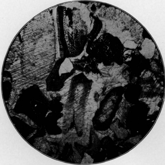
FIG. 1. PHOTO-MICROGRAPH SHOWING LEAN PIECE OF ORE WITH FRAGMENTS OF FOSSILS ONLY PARTIALLY ALTERED INTO IRON OXIDE. Magnified 75 Diameters.
