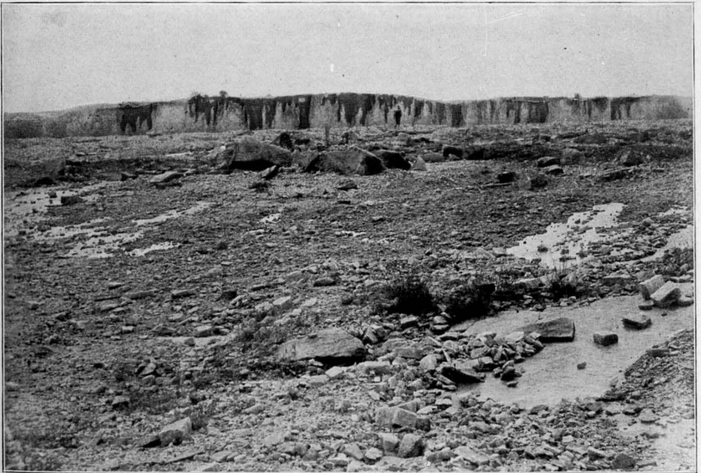
GRANITE-GNEISS QUARRIES, PINE MOUNTAIN, LITHONIA, GEORGIA. FIG. 2 SHOWS THE QUARRY-FACE AND THE QUARRY BOTTOM AT THE SURFACE OF THE DOMING MASS.
