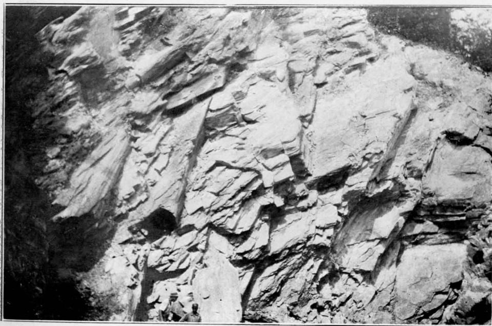
B. ROCKMART SLATES. QUARRY OF ELLIS DAVIS' SONS, ROCKMART, POLK COUNTY, GEORGIA, SHOWING CLEAVAGE. BEDDING NOT SHOWN
