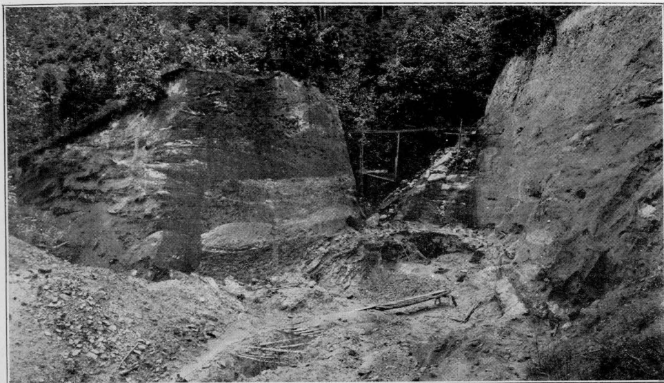
A. VIEW OF THE SALL MOUNTAIN COMPANY'S MINE ON SALL MOUNTAIN, WHITE COUNTY, SHOWING OVAL SHAPED ASBESTOS BODY OVERLAIN BY DECOMPOSED GNEISS.
