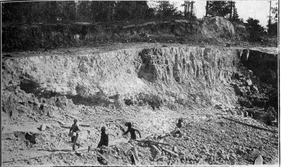
A. CLAYMONT KAOLIN MINE, WILKINSON COUNTY. THE PROJECTING BED IS A LENS OF NODULAR, SLIGHTLY INDURATED CLAY.
