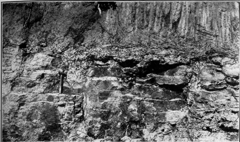
A. WORKING FACE IN THE McINTYRE BAUXITE MINE OF THE REPUBLIC MINING & MANUFACTURING CO., SHOWING BEDDED BAUXITE WITH AN UNCONFORMITY ABOVE.
