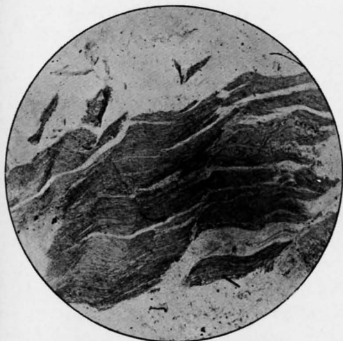
A. SECTION S-210. SERICITE SCHIST FROM LOT 119, SHOWING FOLDING OF THE ORIGINAL CLEAVAGE PRODUCING SECONDARY OR FALSE CLEAVAGE, TRANSMITTED LIGHT. MAGNIFIED ABOUT 13 DIAMETERS.
