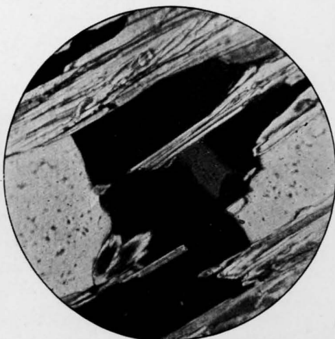
D. SECTION 71. QUARTZITIC SERICITE SCHIST. SHOWING RECRYSTALLIZED QUARTZ GRAINS CUT BY PLATES OF SERICITE. CROSSED NICHOLS. MAGNIFIED ABOUT 130 DIAMETERS.
