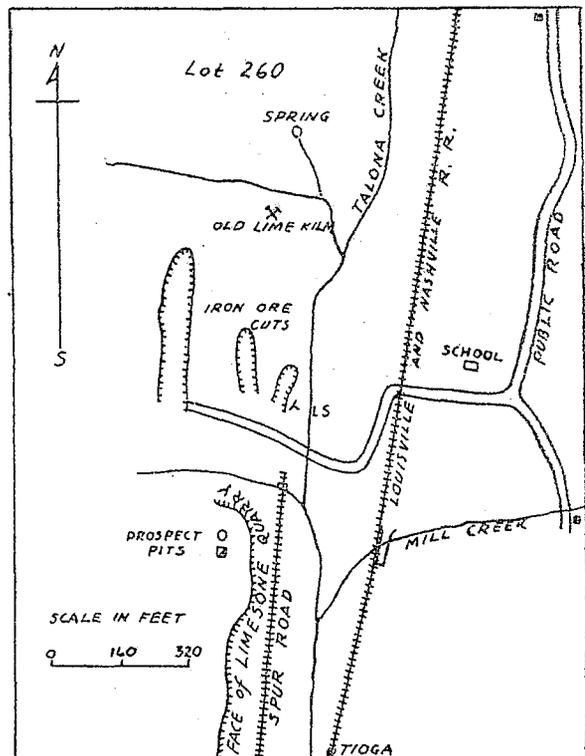
Fig. 5. Sketch map of Ga. Tioga Iron Company's mine at Tioga, Gilmer Co. Ga. (J. P. D. Hull)
