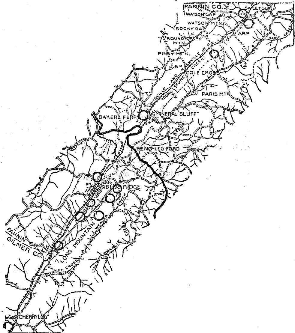
Fig. 4.—Sketch map of part of Fannin and Gilmer Counties showing distribution of iron ore. The circles indicate the locations of main ore deposits.
