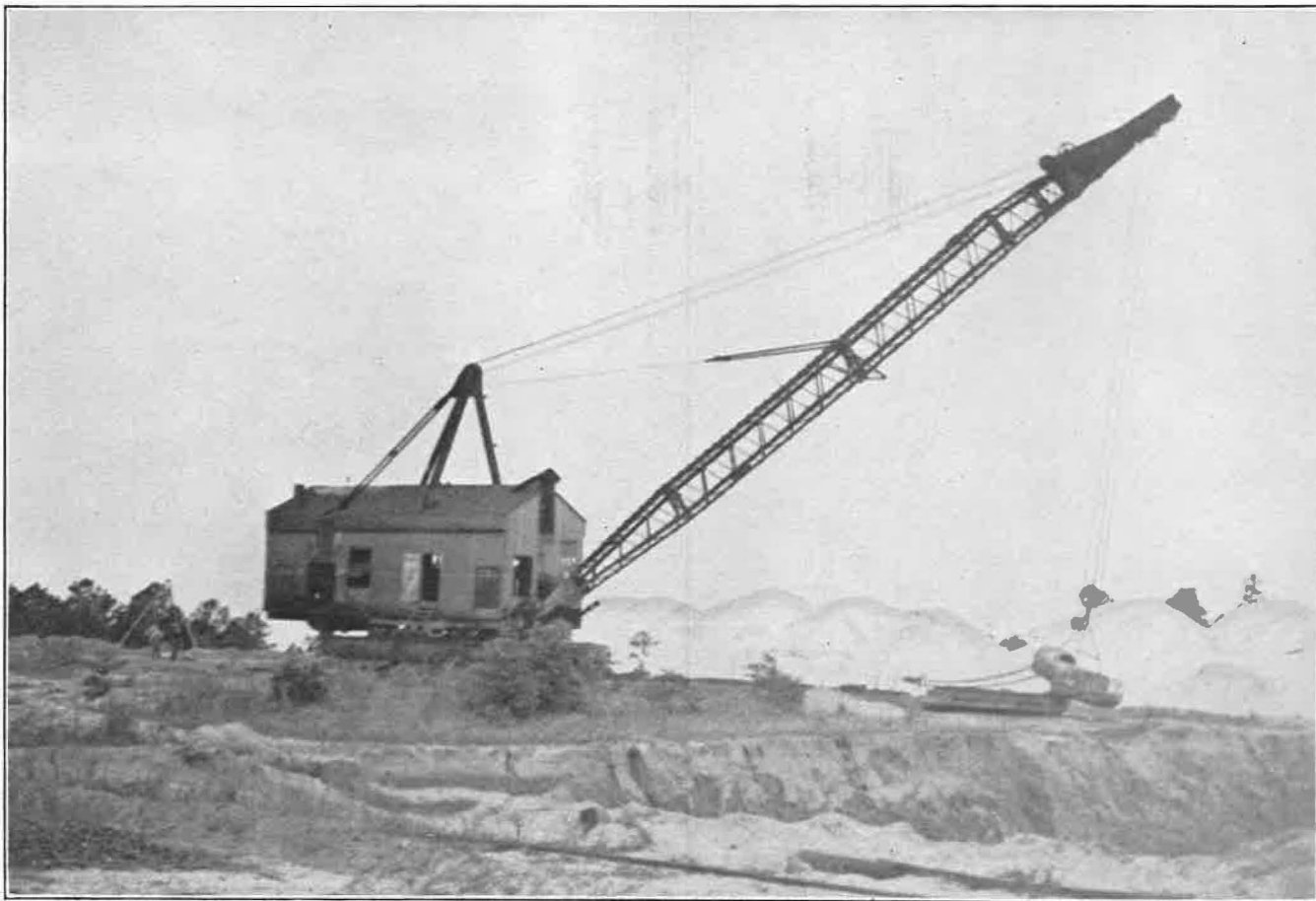
MOVABLE DRAGLINE SCRAPER OWNED BY P. W. MARTIN, GORDON CLAYS, INC. THIS MACHINE IS USED TO REMOVE OVERBURDEN.
