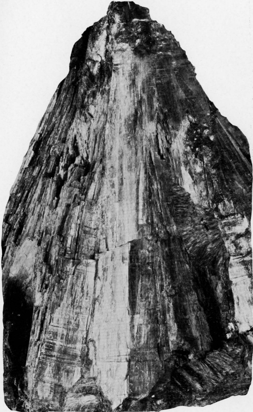
MASSIVE KYANITE FROM GUMLOG, ABOUT 7 MILES NORTH OF BLAIRSVILLE. SHOWING THE CLEAVAGES OF KYANITE AND RADIAL CRYSTALLIZATION FROM A MASS OF CORUNDUM AT THE APEX. NATURAL SIZE.
