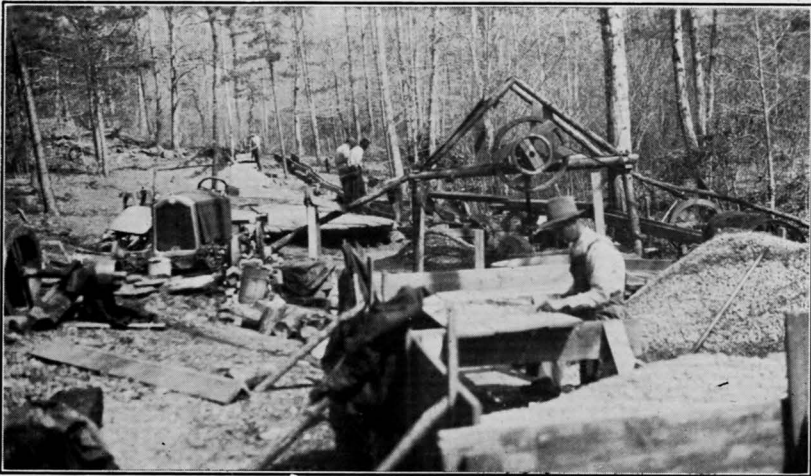
B. PICKING TABLE AND KYANITE WASHER SHOWING PILE OF KYANITE CRYSTALS, ALEC MOUNTAIN, HABERSHAM COUNTY. GEORGIA-CAROLINA MINERALS CORPORATION.
